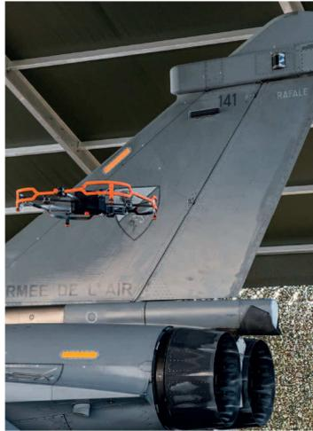
Figure 1: Demonstration of Rafale aircraft inspection by a mini-drone [2]
