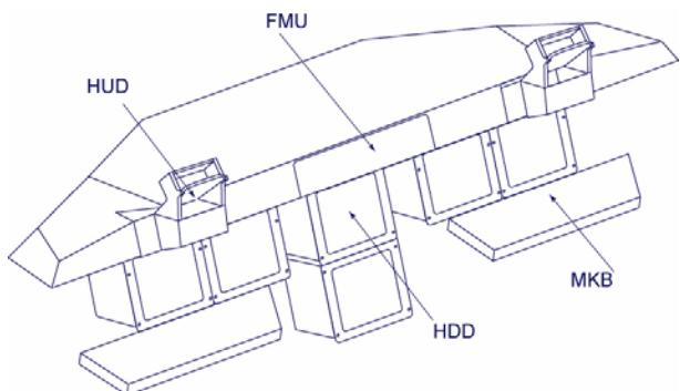
Because of HDDs internal components reached high temperatures leading to a degradation of their performance to provide the vital information required by pilots for a safe return to Earth (in emergency conditions) within 3 hours, two thermal controls were investigated:
