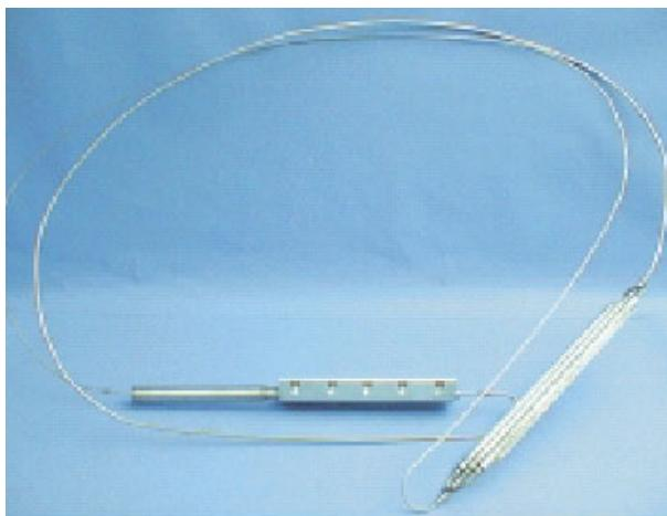
avoiding the high mass, electrical power and induced vibrations of a conventional liquid pump. The loop is able to transport up to 1 kW over a distance of several meters. Due to the extremely small size of the capillary pump, the heat transport against gravity is possible and efficient.
