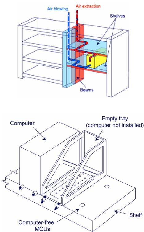
Air blowing and/or air extraction help for dissipating computer heat. Nevertheless, in case of ventilation failure, the equipment is working under the natural air convection. Additionally, for power supply, the use of power bus-bar contributes to the heat internal dissipation in the vehicle.
