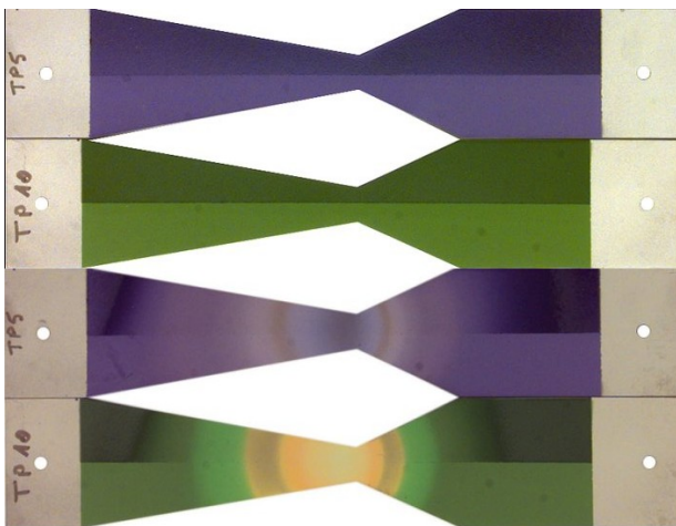
Fig. 4: Other thermal paints before (top) and after heating (bottom)
