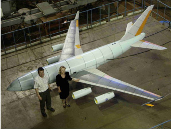
Fig. 1. Aeroelastic wind tunnel model of the long range transport aircraft “EuRAM”
