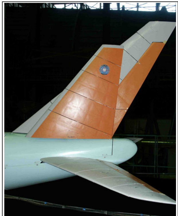
Fig. 13. Tested all-movable vertical tail versus conventional fin with rudder, size comparison on EuRAM empennage
