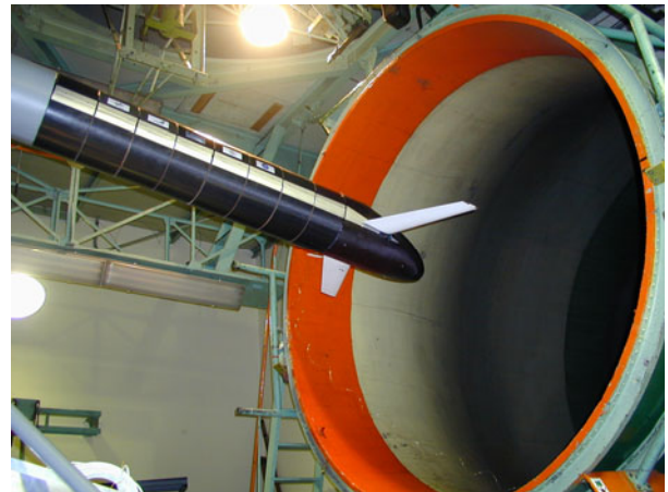
Fig. 16. X-DIA fuselage component with forward swept foreplanes in wind tunnel
