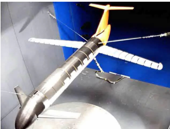
Fig. 15. Complete X-DIA wind tunnel integration
