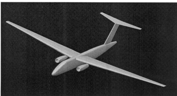
Fig. 3. High aspect ratio wing “HARW” for a HALE-UAV
