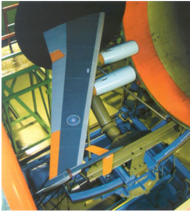
Fig. 7. Right EuRAM half wing in VZLU wind tunnel, arrow AWTC installed in-plane at tip chord
