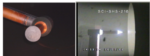
Fig. 4. SHS Nose_0 before and during the test
