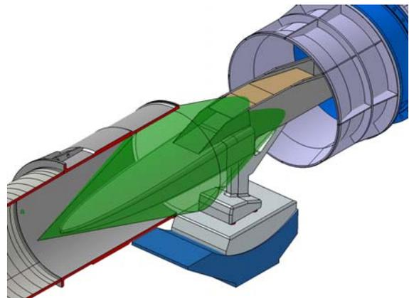
Fig. 11 – Study of LEA free-jet test installation in S4Ma ONERA test facility
