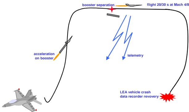
Fig.2 –LEA flight testing sequence
