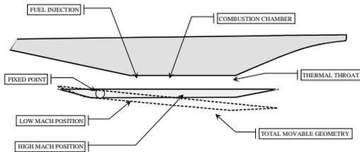
Fig.5 – variable geometry PROMETHEE engine
