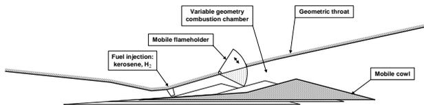
Fig.6 – variable geometry PIAF engine
