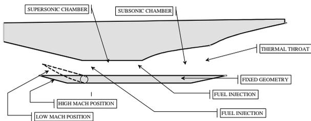
Fig.4 – fixed geometry JAPHAR engine
