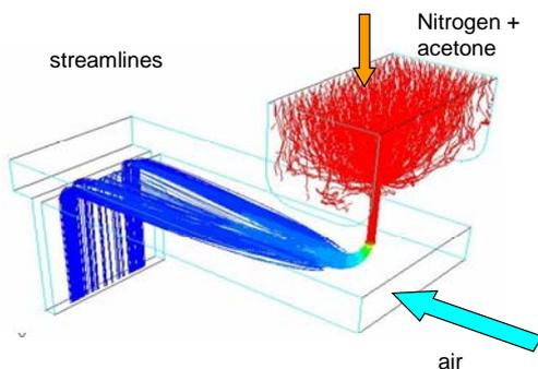
Fig. 6 : Premixed channel (FLUENT simulation)
