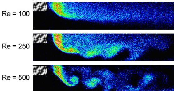
Fig. 8b : Flow images with turbulence promoters upstream from the injection
