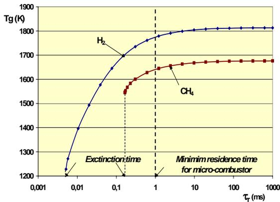
Fig. 4 : Gas temperature versus residence time for H<sub>2</sub> and CH<sub>4</sub>
