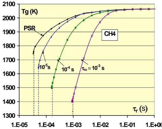
Fig. 3 : Gas temperature versus residence time for different mixing time scales (without heat loss)
