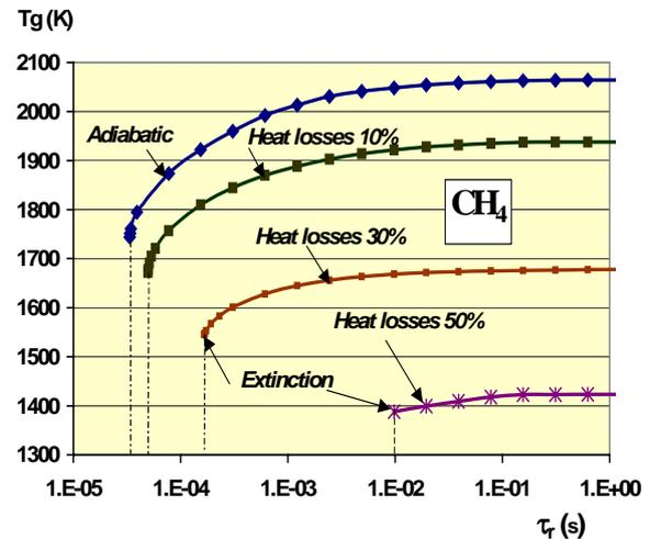
Fig. 2 : Gas temperature versus residence time for different levels of heat losses
