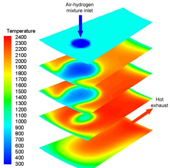
Fig. 5a : Gas temperature inside a sector of the micro-combustor – ONERA CFD code
