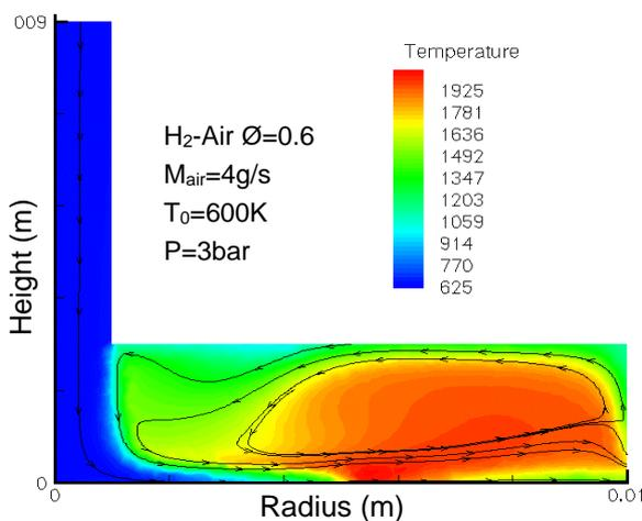
Fig 10 : Computation of gas temperature in the combustion chamber (CEDRE)
