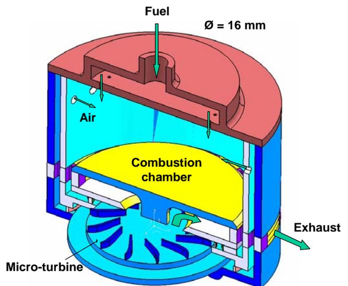
Fig. 11 : Alternative design of micro-turbine (external diameter : 16 mm)
