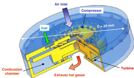
Fig. 1 : 3D representation of micro-turbine MITconcept
