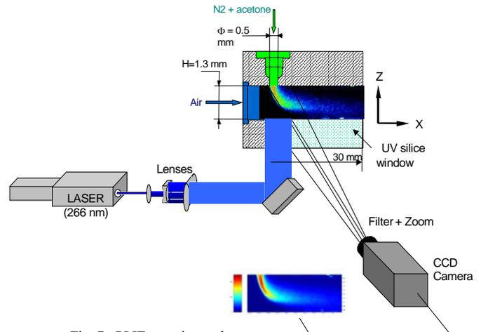
Fig. 7 : PLIF experimental set-up
