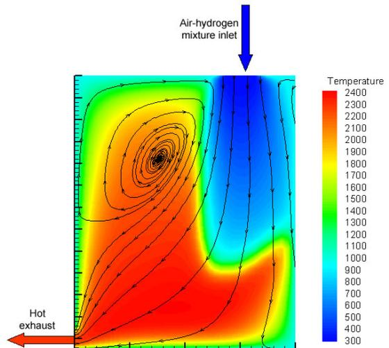
Fig. 5b : Streamlines and gas temperature in a cross-section of the combustor
