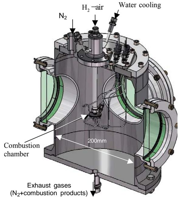
Fig. 9a : Set-up for combustion tests
