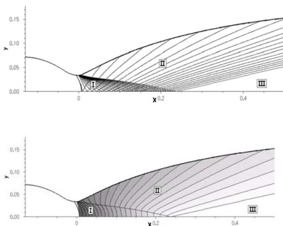
Fig. 7. Flow regions in a TIC nozzle: (a) Characteristic line net, (b) Mach number isolines
