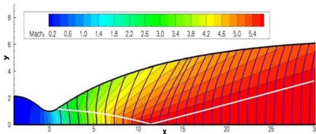
Fig. 8. Approximated shock profile reconstruction in a TIC nozzle
