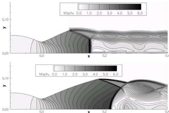
Fig. 5. Inviscid simulations with flat and curved Mach stem. (a) PR=10, (b) PR=20
