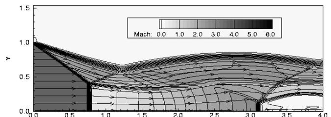
Fig. 4. Inviscid simulation with uniform incoming flow and classical Mach reflection
