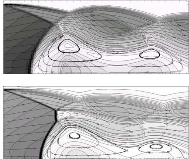
Fig. 6. Comparisons of viscous and inviscid results: (a) Inviscid flow, (b) Viscous laminar flow
