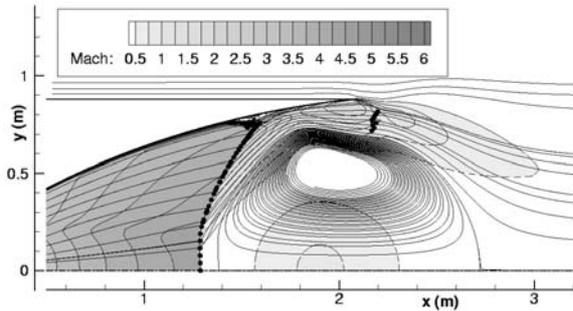
Fig. 2. The role of the centreline vortex in generating Restricted Shock Separation regimes
