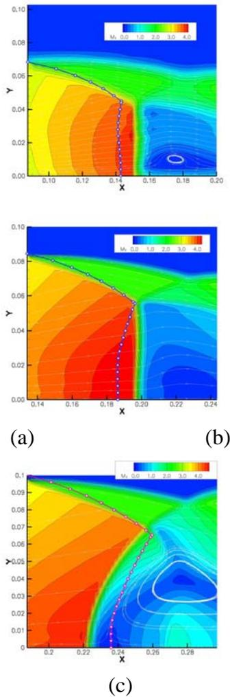
Figure 9. Analytical and numerical predictions of the shock shape for a separated TIC nozzle flow:
