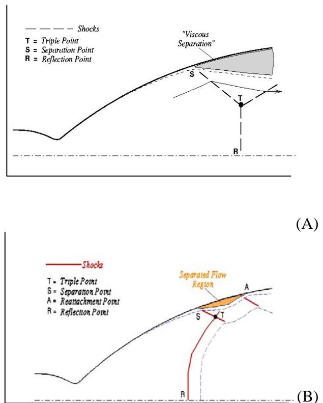
Fig. 1. Free (A) and Restricted (B) Shock Separation regimes
