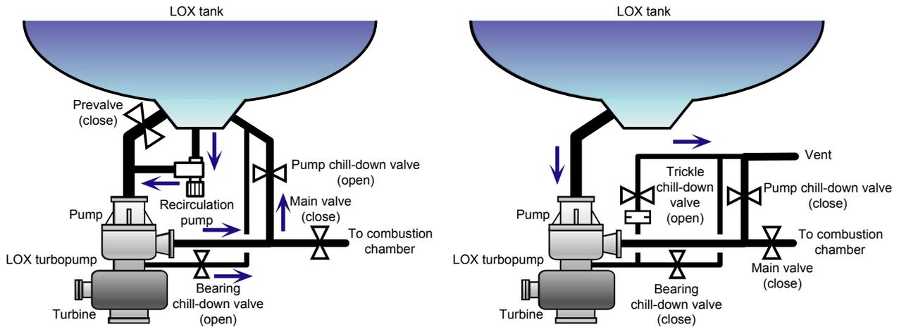
Figure 8: Schematics of recirculation chill-down system (left) and trickle chill-down system (right).
