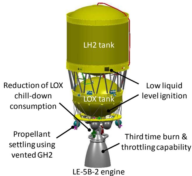
Figure 6: Upper stage propulsion system of H-IIA and development items for H-IIA upgrade.
