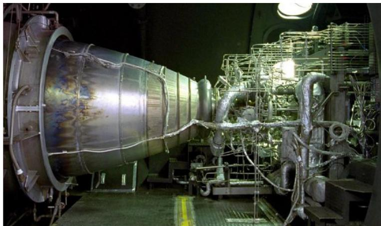
Figure 7: LE-5B-2 upper stage engine in HATS (High Altitude Test Stand).
