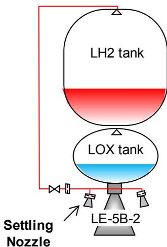
Figure 9: Schematic of GH2 vent settling system.
