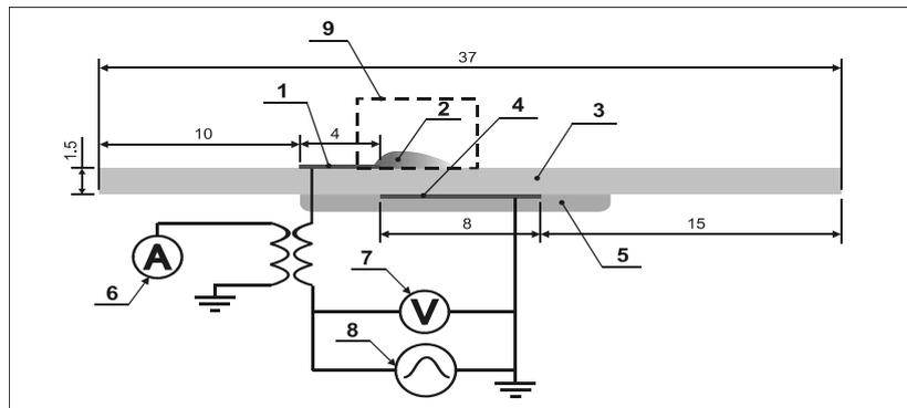
Figure 1 Scheme of DBD (1 – open electrode, 2 – plasma region, 3 – glass-fiber laminate, 4 – closed electrode, 5 – epoxy resin, 6 – current probe, 7 – voltage probe, 8 – high-voltage source, 9- region of PIV measurements)
