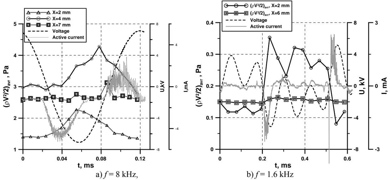
Figure 5 Variation of the dynamic pressure, voltage and plasma current
