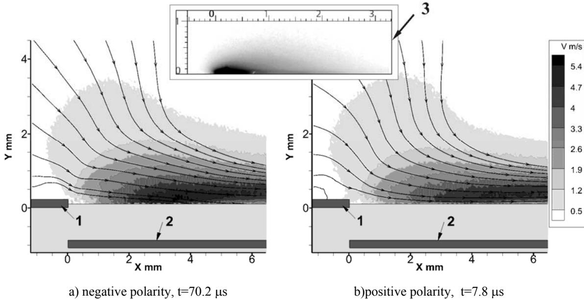
Figure 4. Induced velocity fields at the moment of plasma collapse (1 – exposed electrode, 2 – closed electrode (grounded), 3 – inverted photo of plasma region).
