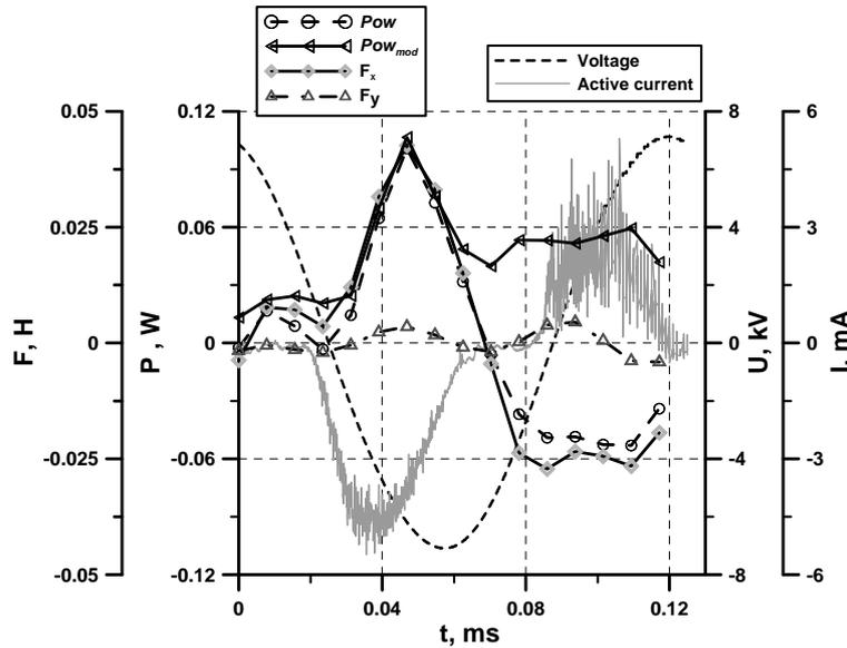
Figure 6 Variation of power during one period on the background of active current and voltage.
