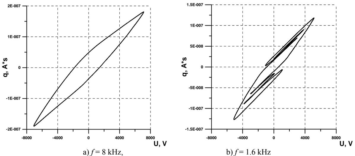
Figure 3. Cyclograms of the voltage and charge variation on DBD a) 8 кГц, b) 1.6 кГц
