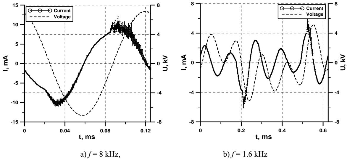
Figure 2. Oscillograms of voltage and current measured on DBD
