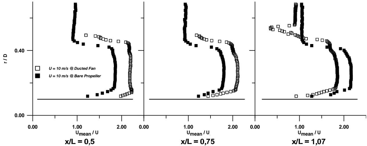
Figure 10: Comparison of Velocity Profiles inside the slipstream of bare propeller and inside duct,  $N=7000$  rpm and  $U=10$  m/s
