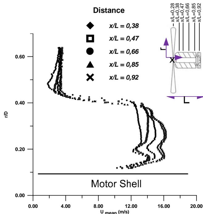
Figure 2: Velocity Profiles at Exit Plane at Static Situation
