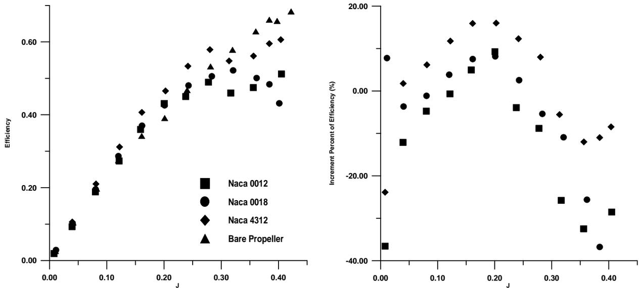
Figure 7: Figure of Merit and % increment of efficiency at 7000 rpm Rotor Speed
