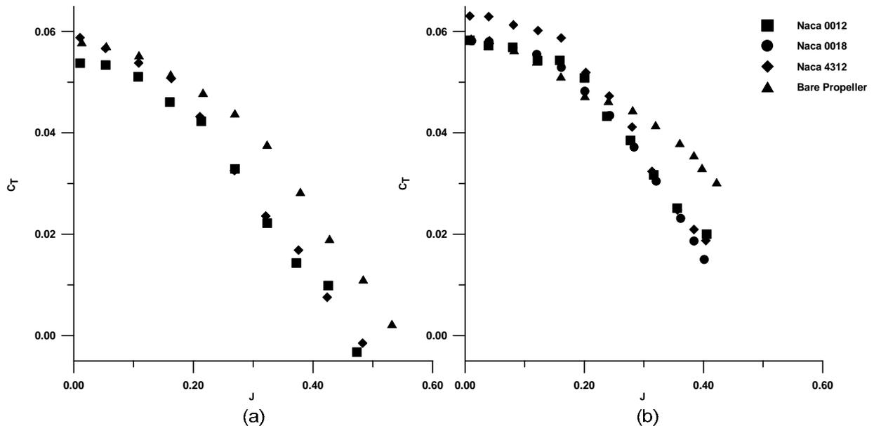
Figure 6: Thrust Coefficient versus Advance Ratio at (a) 5300 rpm, (b) 7000 rpm
