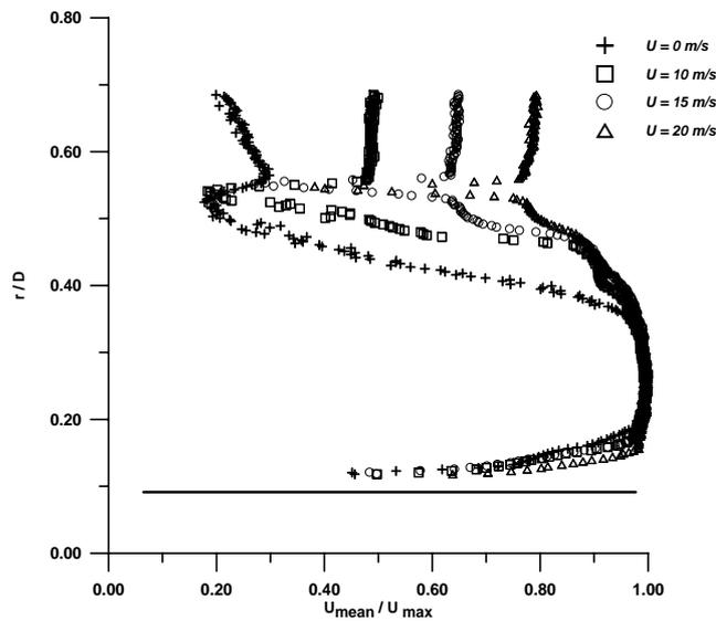
Figure 9: Velocity Profiles at Exit Plane of NACA 4312 Duct  $N=7000$  rpm
