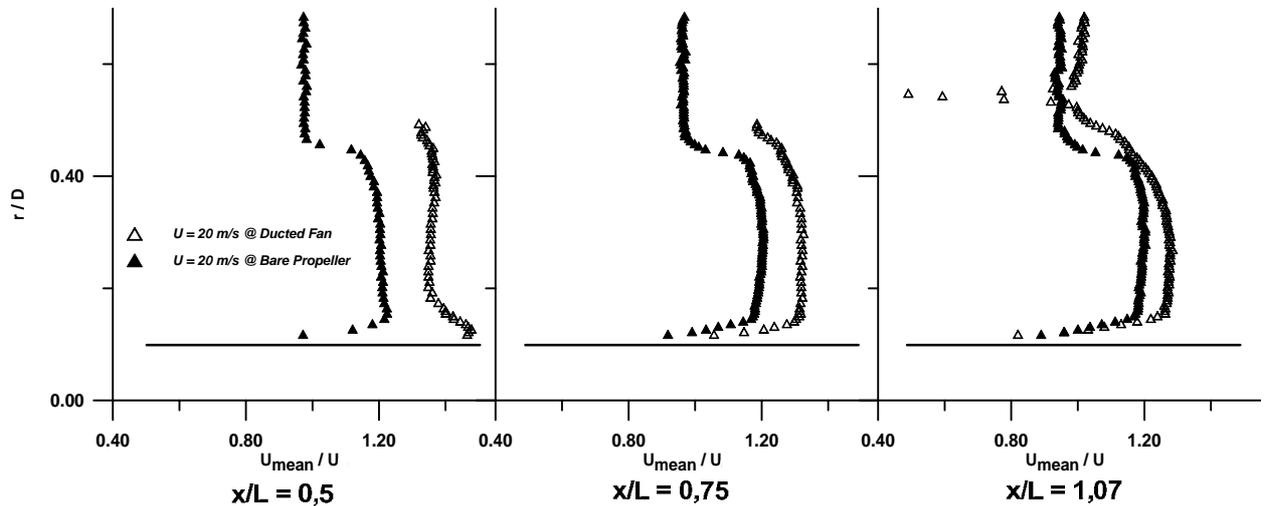
Figure 11: Comparison of Velocity Profiles inside the slipstream of bare propeller and inside duct,  $N=7000$  rpm and  $U=20$  m/s
