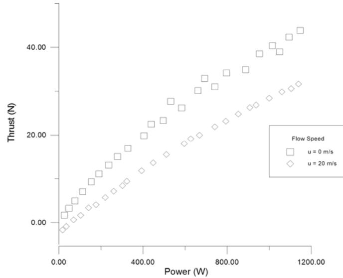
Figure 3: Thrust Produced by Open Propeller
