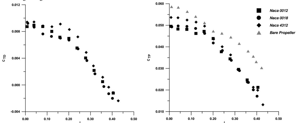
Figure 4: Thrust components produced by duct and propeller (N=7000rpm)
