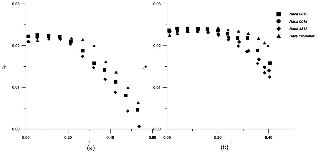
Figure 5: Power Coefficient versus Advance Ratio at (a) 5300 rpm, (b) 7000 rpm
