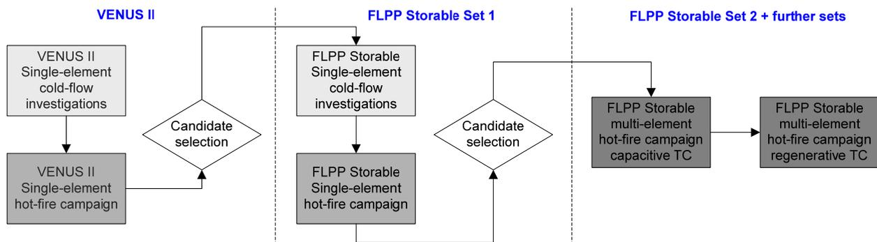
Figure 3: Injection technology development logic
