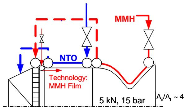
Figure 4: FLPP Storable cooling architecture
