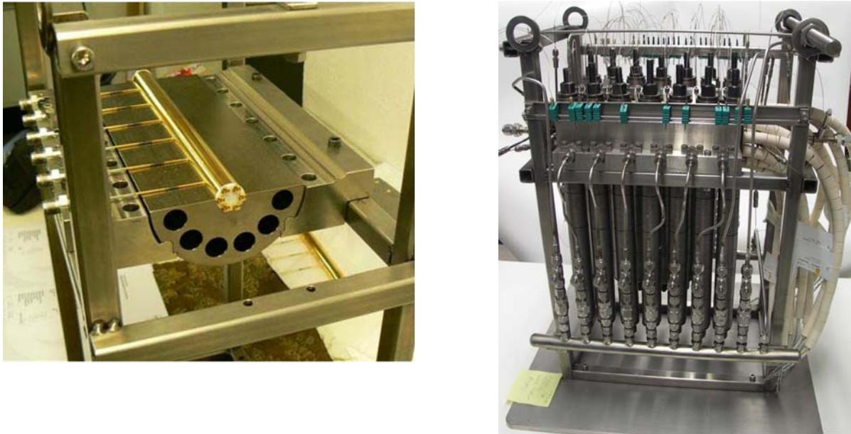
Figure 6: EHT modular setup with gold-plated nickel tube (left); side view of mounted setup (right);
