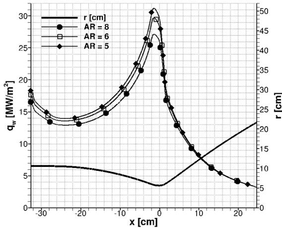
Figure 9: Wall heat flux.
