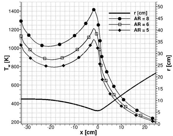
Figure 10: Hot-gas side wall temperature.
