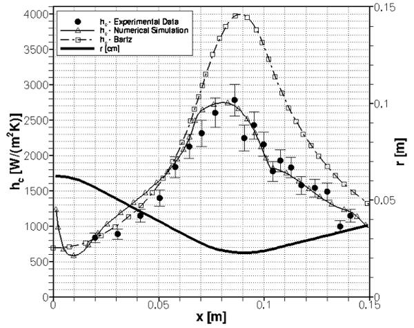
(b) Comparison between experimental data, CFD numerical solution and Bartz's semi-empirical model.
