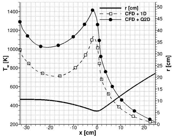
Figure 8: Hot-gas side wall temperature.
