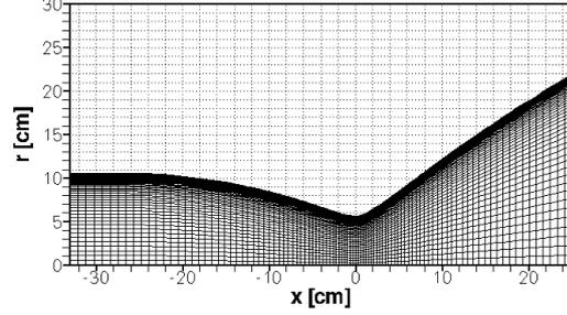
Figure 4: Numerical grid for the hot gas flow simulation.
