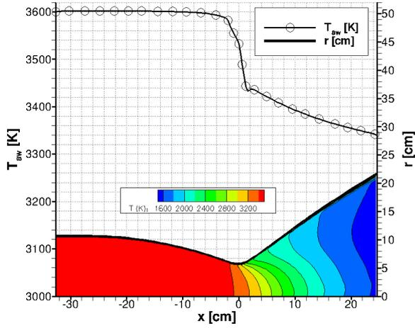
Figure 5: Wall temperature and temperature field in the nozzle in case of adiabatic wall.
