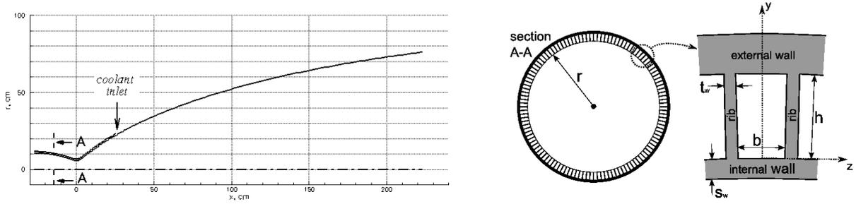
Figure 2: Schematic of nozzle and regenerative cooling channels.
