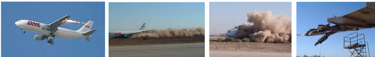
Figure 1: Emergency landing sequence using engines only and left wing structural damage due to surface-to-air missile impact, DHL A300B4-203F, Baghdad, 2003
