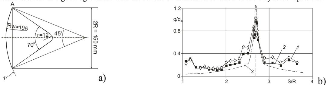
Figure 3: Heat exchange in the bottom part of the Martian probe schematic model at  $M_\infty = 8, Re_{\infty,D} = 1 \times 10^6$ : 1 – without turbulator; 2 – with the turbulator, placed on the frontal surface; 3 – calculation.  $q_0$  – heat flux in the frontal point of stagnation,  $D=2R$  – overall size of the model,  $S$  – contour length from the arm.
