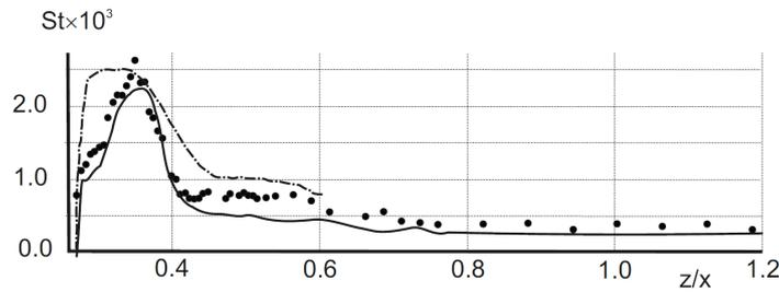
Figure 5: Stanton number distribution on a plate in the cross-section, situated at distance  $x = 82$  mm from the wedge leading edge ( $x/L = 0.46$ ), at  $M_\infty = 5$ ,  $Re_{xL} = 27 \times 10^6$  and wedge angle  $\theta = 15^\circ$ : solid line – TSP, points – thermocouples, dash-and-dot line – calculation.
