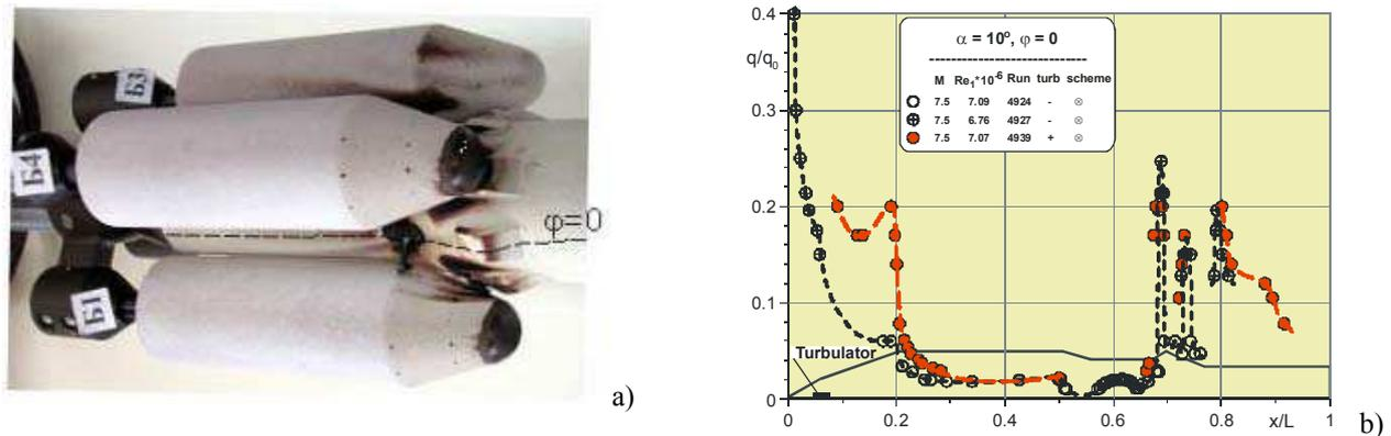
Figure 2: Investigation of the heat exchange distribution over the “Angara” model surface in T-117. a) Photo of the model after tests b) a) Distribution of Stanton number  $St$  along model length  $x/L$  at the azimuthal angle  $\varphi = 0/$
