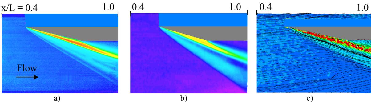
Figure 4: Flow over a flat plate with a wedge of  $\theta = 15^\circ$  at  $M = 5$  and  $Re_{\infty,L} = 27 \times 10^6$ : a – distribution of the Stanton number; b – distribution of pressure ratio  $C_p$ ; c – limit streamlines and friction stress.
