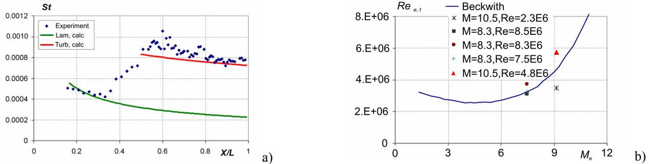
Figure 1: Investigation of a laminar-turbulent transition on a sharp cone with an angle of a half-expansion of  $5^\circ$  in T-117 wind tunnel.  $M_\infty=10.5$ ;  $M_e=8.3$ ; a) Distribution of the Stanton number along model length  $x/L$ .  $M_\infty=8.3$ .  $Re_{\infty,L}=9.04 \times 10^6$ . b)  $Re_{e,t} = f(M_e)$ .
