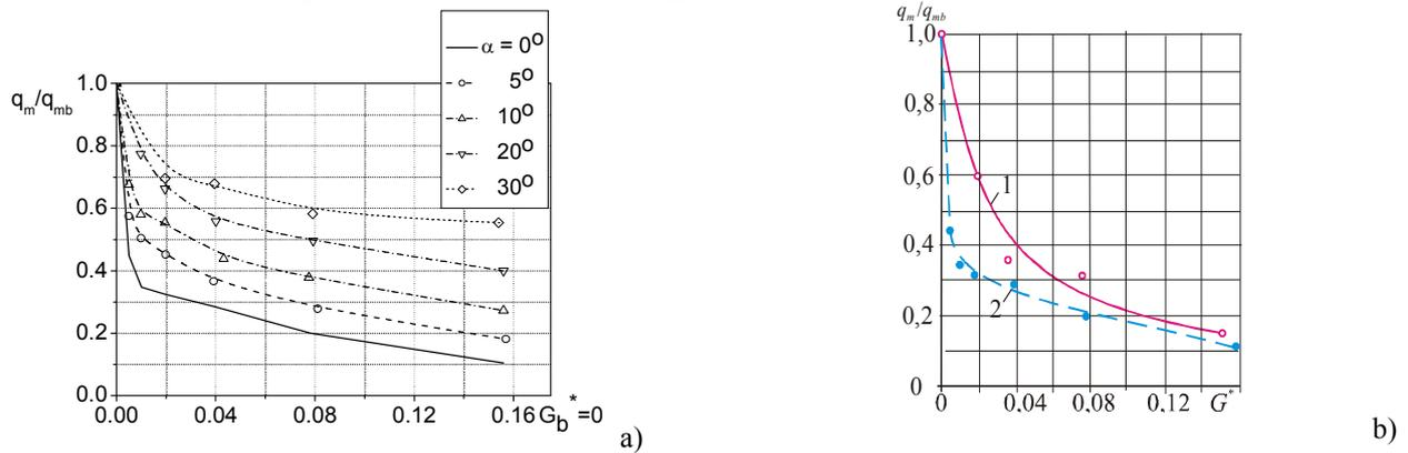
Figure 6: Influence of injection gas flow  $G^*$  on the maximum heat flux to the blunting surface. a) at different angles of attack  $\alpha$  of the cylinder . b) at different concentrations of particles in the undisturbed flow. 1 –  $n = 1.6\%$ , 2 –  $n = 0$ .  $n$  - the weight concentration of particles  $Fe_2O_3$  size  $d = 0.37$  mkm.
