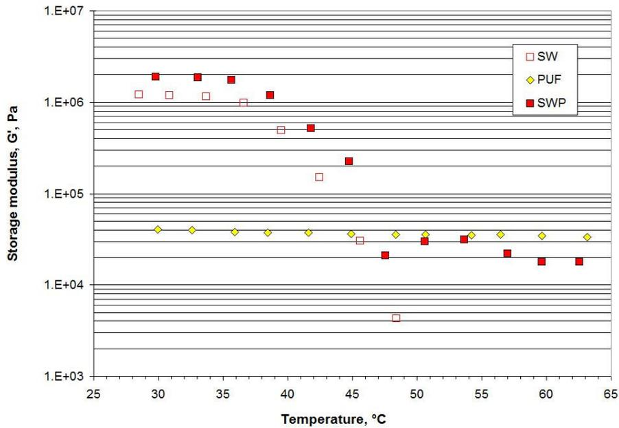
Figure 4: Storage modulus vs. temperature in a parallel-plate rheometer for SW, SWP and PUF. Strain =1%.
