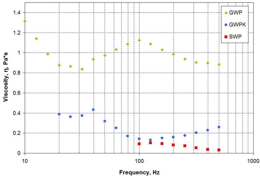
Figure 2: Measured viscosity (by Couette viscosimeter) of GW, SW and GW added with KER, showing the effect of kerosene addition and the very low viscosity of the melted SW, which is responsible for a large entrainment effect. Tests were performed at 70 °C.
