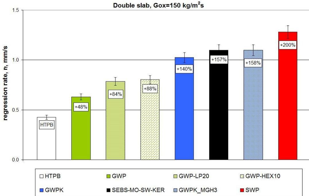
Figure 7: Regression rate comparison for different fuel formulations.
