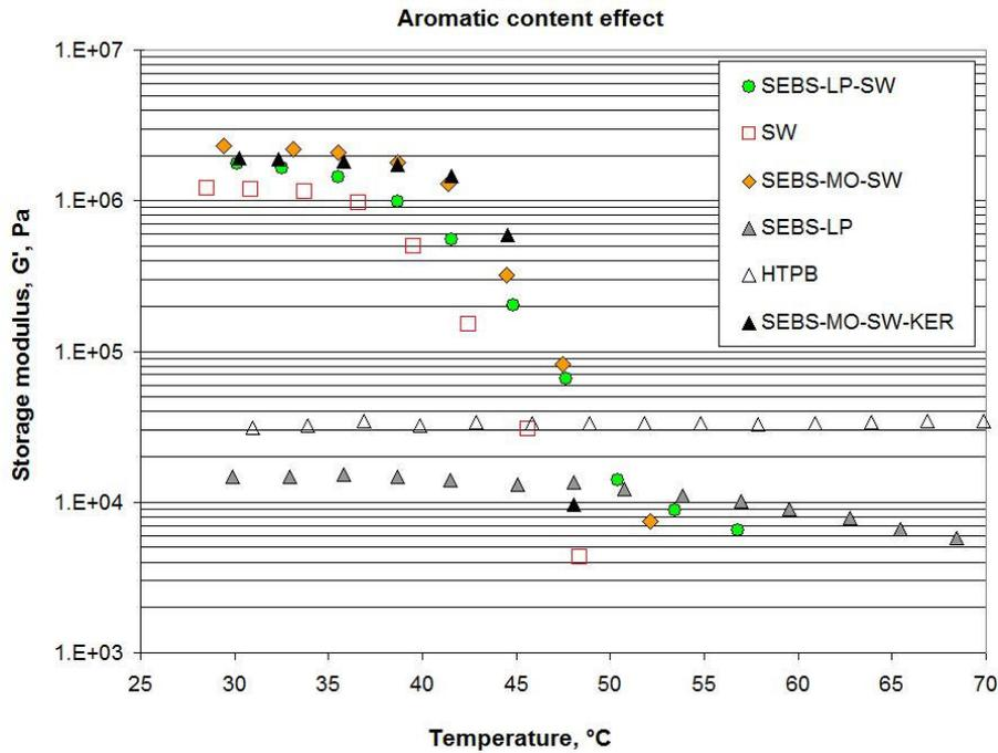
Figure 5: Storage modulus vs. temperature in a plate-plate rheometer for SEBS-containing fuel formulations. Strain=1%.
