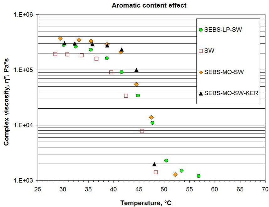
Figure 6: Complex viscosity vs. temperature for SEBS-containing formulations. Strain=1%.
