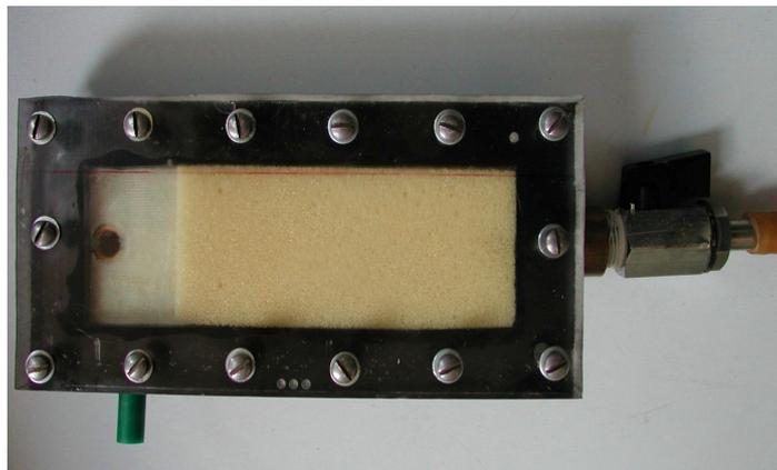
Figure 1: Sample mould and PUF strengthening structure for paraffin-based fuel formulations.
