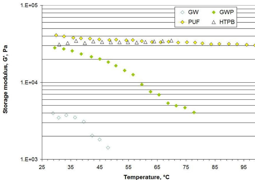
Figure 3: Storage modulus vs. temperature in a parallel-plate rheometer for GW, GWP and PUF. HTPB is shown as a reference value. Strain = 5%.
