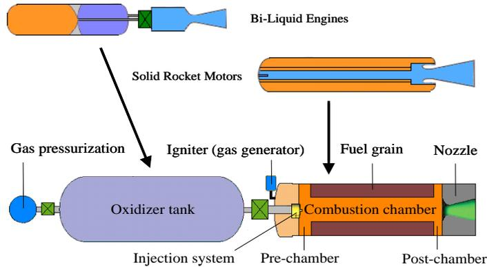
Figure 1: Hybrid propulsion concept
