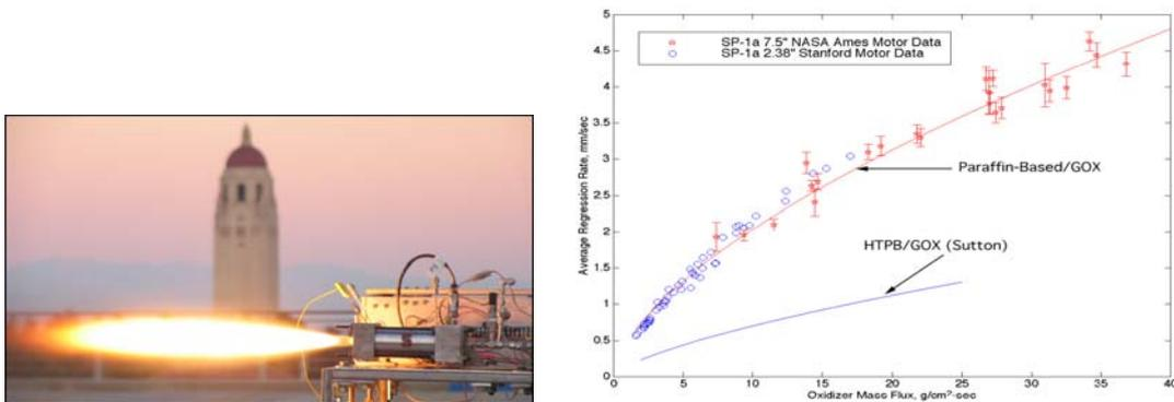
Figure 12: Hot fire test at Stanford University and comparison of regression rate for paraffin-based and HTPB fuels
