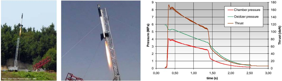
Figure 8: Flight test of the FH-01 rocket at La Courtine (PE / N<sub>2</sub>O)
