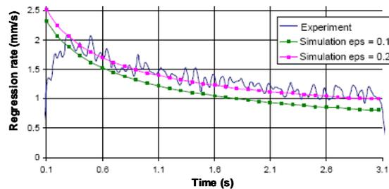
Figure 10: Instantaneous regression rate comparison between DEPHY results and Onera test case
