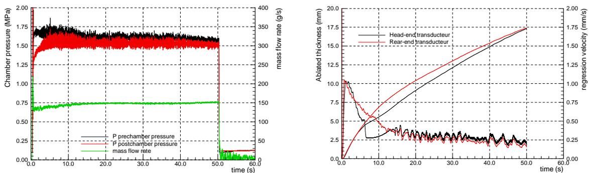
Figure 5: Results for one of the first test using the Onera hybrid motor (PE /  $H_2O_2$ )
