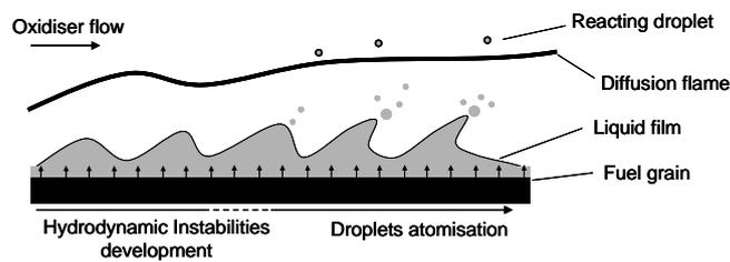
Figure 11: Karabeyoglu’s schematic of entrainment process for liquefied fuels
