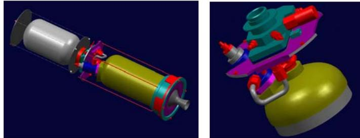
Figure 6: Overview of the FUSEX engine (left) and pyrotechnic valve (right)
