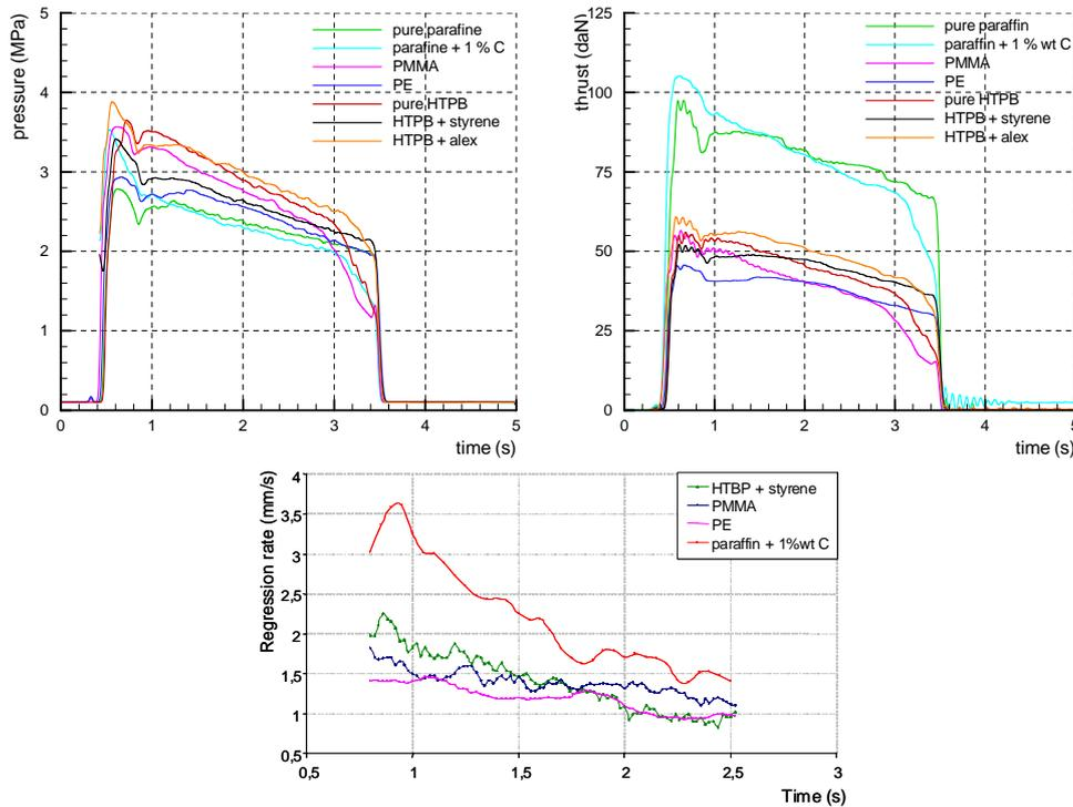
Figure 13: Evolutions of chamber pressure, thrust level and regression rate for different fuel formulations
