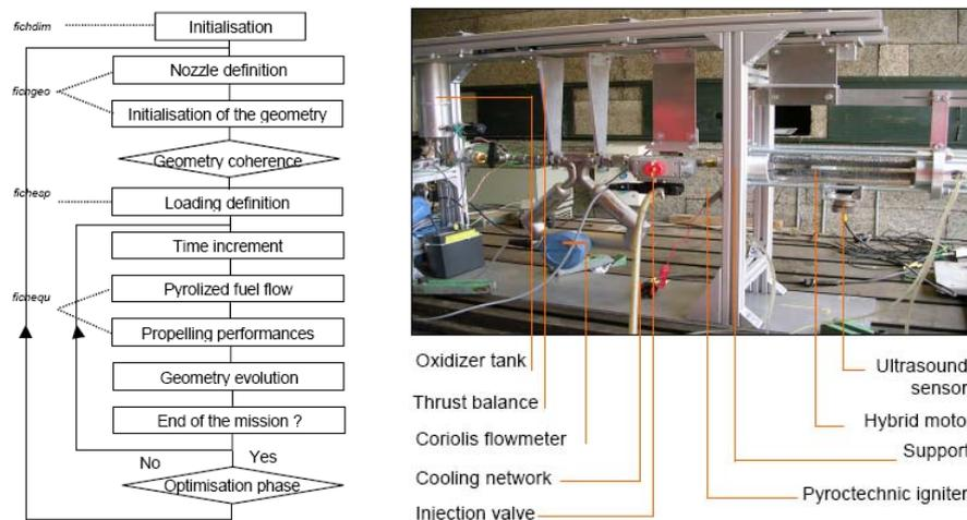
Figure 9: Organization of the DEPHY numerical code (left) and overview of the Onera test facility (right)
