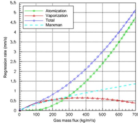
Figure 14: Total regression rate and its contributions in function of the gas mass flux
