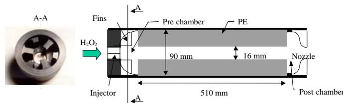
Figure 4: Structure of the first Onera hybrid motor
