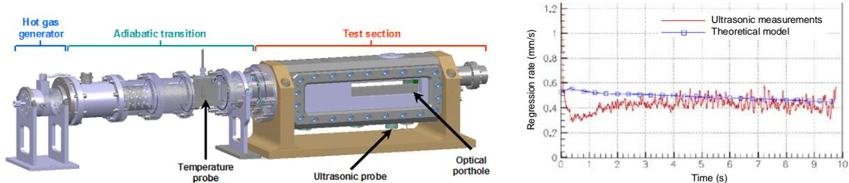
Figure 15: HYPARRE facility and comparison of the measured and computed (0D model) regression rate
