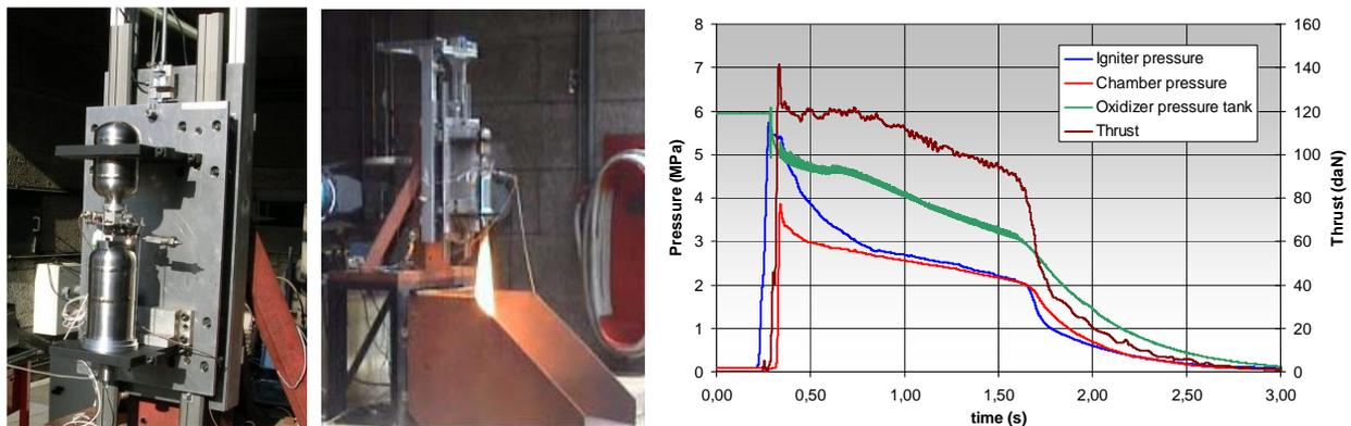
Figure 7: FUSEX engine before the firing and ignited and measurements during ground firing test
