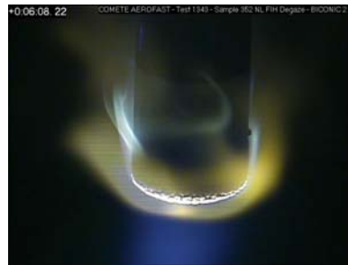
Figure-26: Plasma tests on Cork based material
