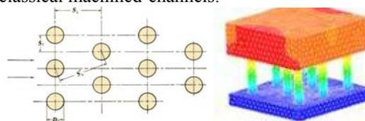
*Figure 1 : pin fin configuration of cooling channel*
