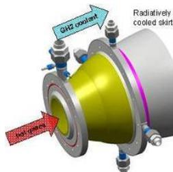
Figure 6 : project of subscale PTAH LRE nozzle extension
