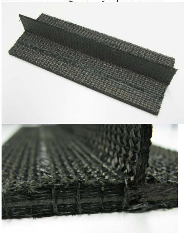
Figure 9 : PTAH SOCAR panel with integrated stiffener at preform state - detail
