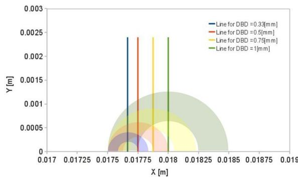
Figure 5: Lines where the pressure values are extracted for each wave.
