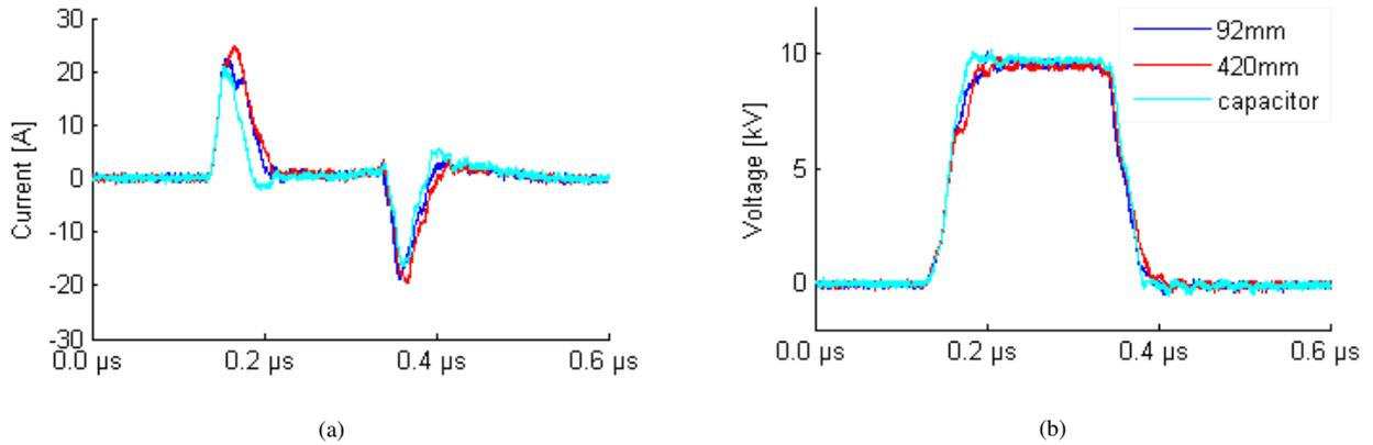
Figure 3: Comparison of current (a) and voltage (b) waveforms acquired with a  $27 \text{ pF}$  capacitor and single DBD actuators with  $92 \text{ mm}$  (actuator 1) and  $420 \text{ mm}$  (actuator 3) electrode length ( $U_p = 10 \text{ kV}$ ).
