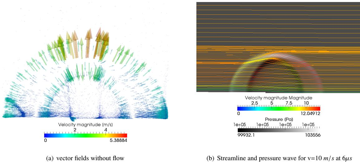
Figure 7: Behaviour of the compression wave
