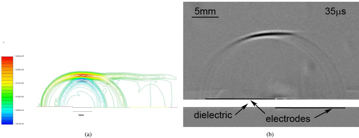
Figure 9: Simulation at  $t=5\mu s$  (a) and phase averaged schlieren images of the compression wave emerging from the surface of actuator 1 without flow ( $U = 10 kV$ ,  $t_w = 200 ns$ ,  $R_s = 33 \Omega$ )(b).
