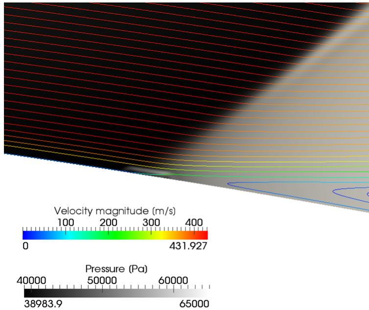
Figure 8: Streamline and pressure fields for the profile Naca3505 at Mach=0.7 in the shock region
