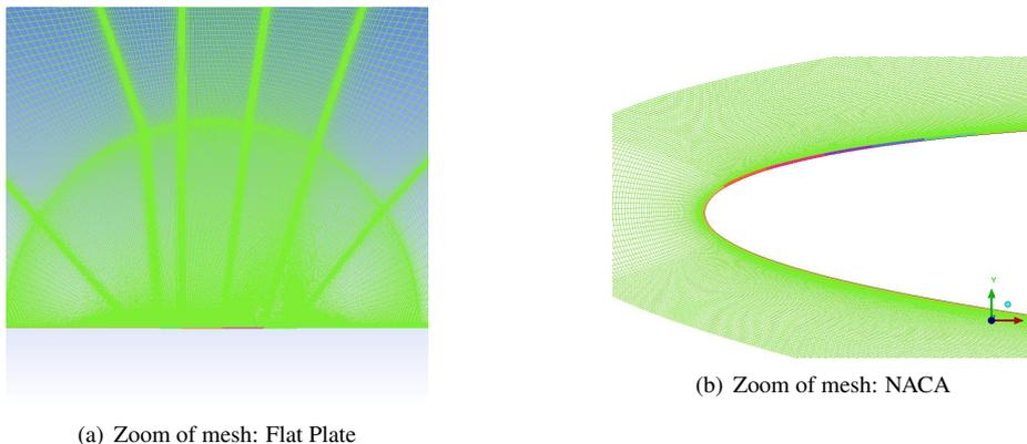
Figure 1: Zoom of the meshes close to the DBD's for the Flat Plate geometry (a) and the NACA3506 (b). The DBD's are indicated by the coloured boundaries.
