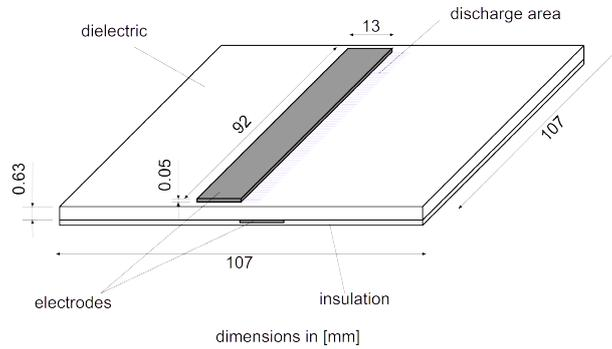
Figure 4: Configuration of the DBD actuator with  $Al_2O_3$  dielectric.
