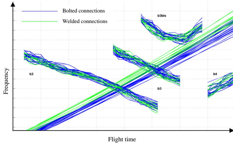
Figure 4: Evolution of SRB longitudinal mode from bolted to welded connections
