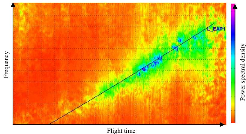
Figure 2: In-flight evolution of the SRB first longitudinal mode
