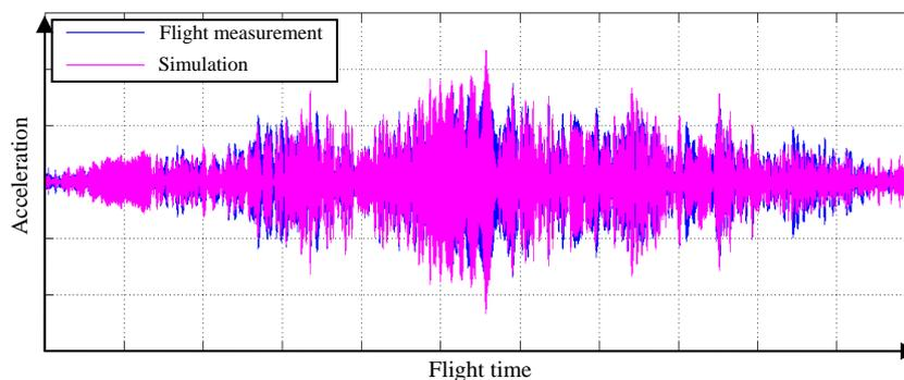
Figure 6: Validation of viscous damping value corresponding to the SRB longitudinal mode
