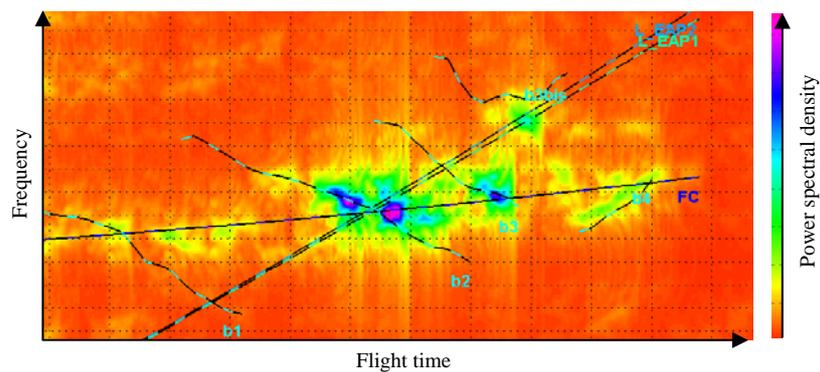
Figure 5: Longitudinal acceleration response at main cryogenic stage oxygen tank lower bulkhead
