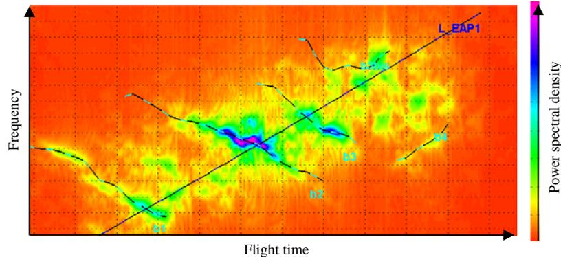
Figure 3: Longitudinal acceleration response of the SRB
