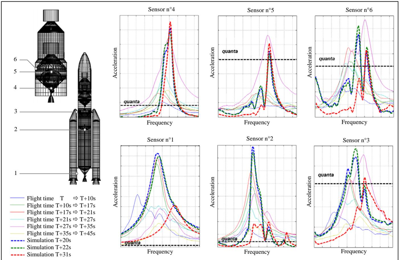
Figure 7: Comparison between simulation results and flight measurements
