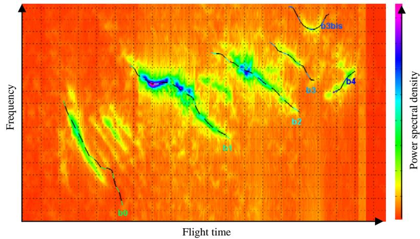
Figure 1: In-flight evolution of SRB internal pressure power spectral density
