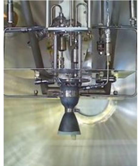
Figure 5: 400 N engine mounted on test stand
