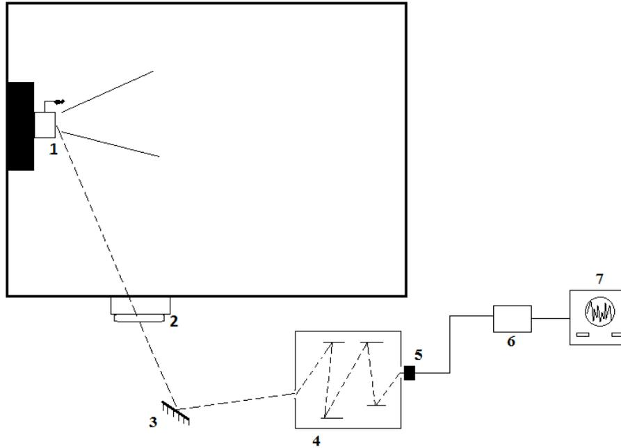
Figure1: Experimental setup: 1 – thruster, 2 – quartz side port, 3 – aluminium mirror, 4 – monochromator, 5 – photomultiplier, 6 – amplifier, 7 – oscillograph
