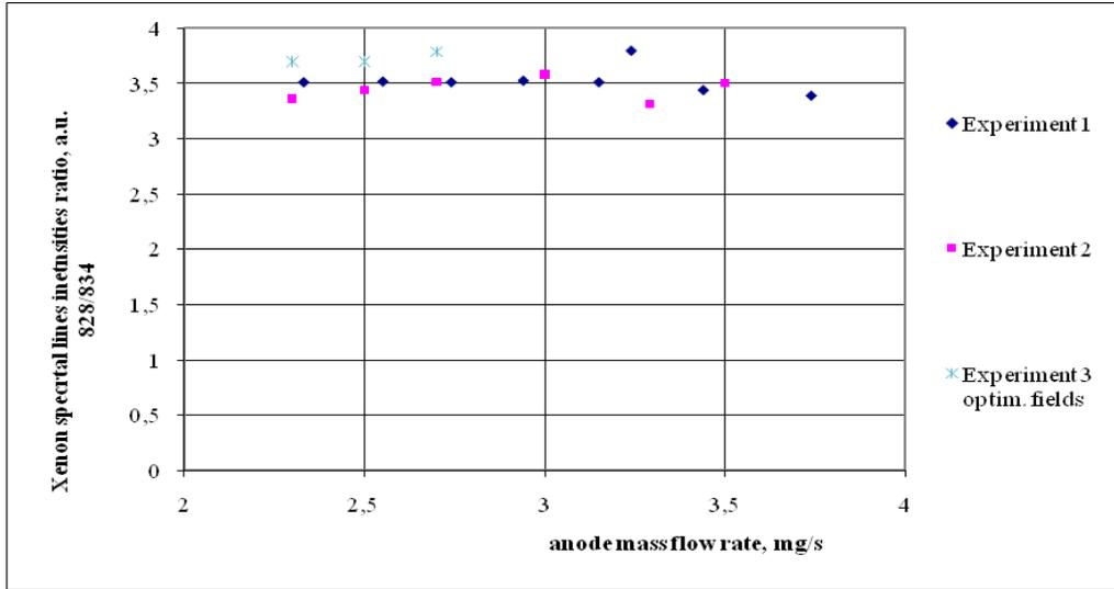
Figure 6: Xenon spectral lines intensities ratio dependency on anode mass flow rate.
