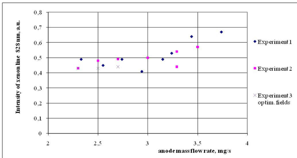
Figure 3: Xe line intensity corresponding to 828 nm
