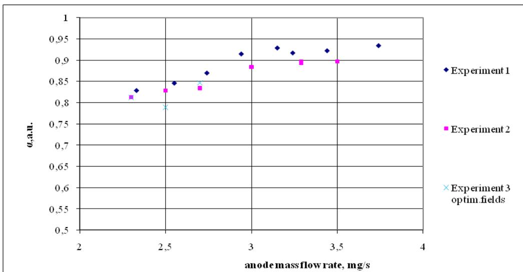
Figure 5: Propellant utilization coefficient dependency on anode mass flow rate.
