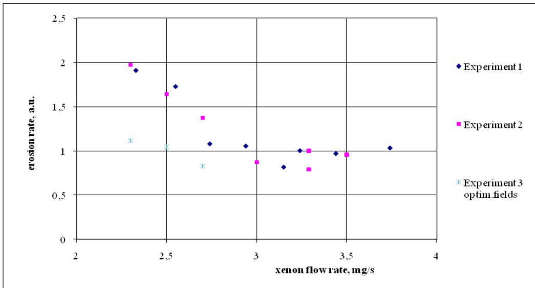
Figure 7: Relative erosion rate in different operation modes.
