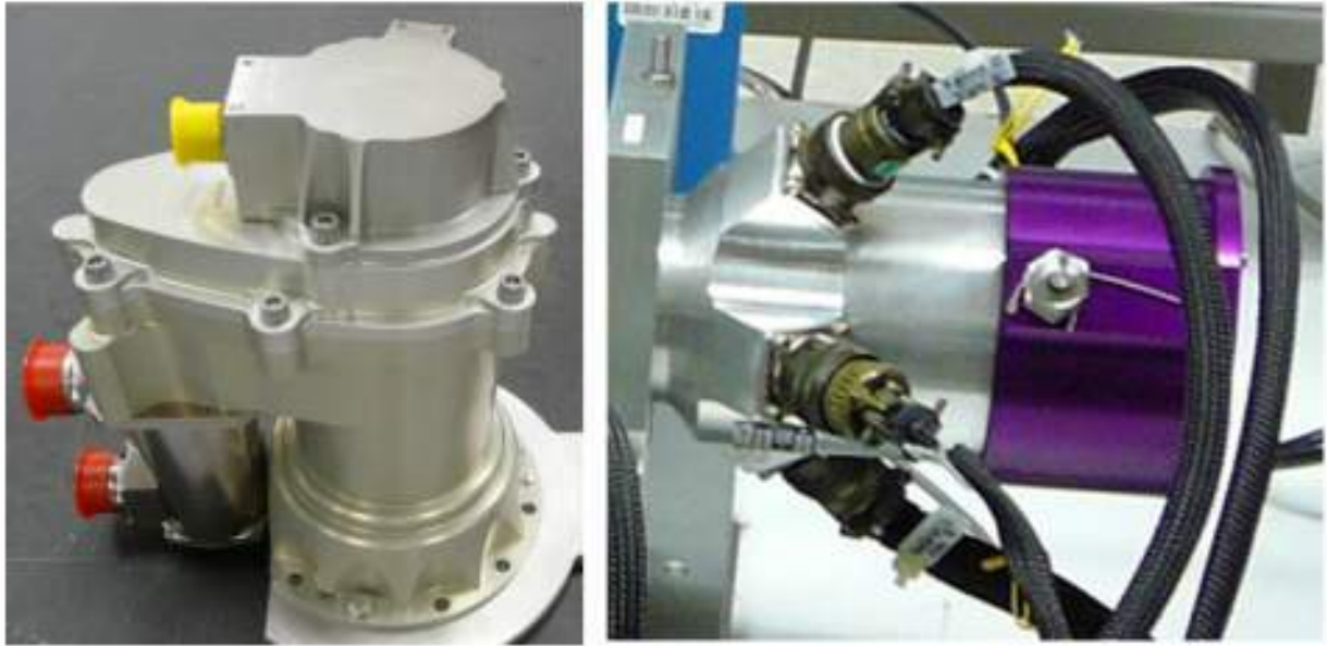
Figure 4 : Hot gas VGC valve and VRR actuator
