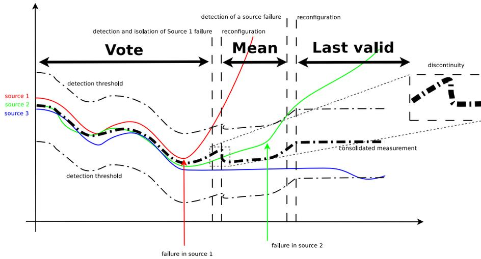
Figure 2: Triplex monitoring
