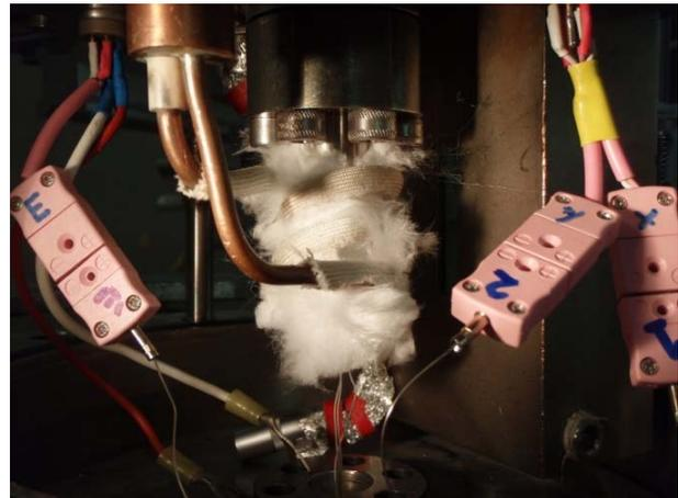
Figure 5 : Picture of the equipment used for the heating of the tensile test sample: the sample is clamped at its top and covered with ceramic wool.
