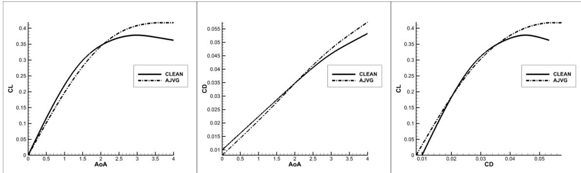
Figure 4. Comparison of polars for AJVG and clean airfoil
