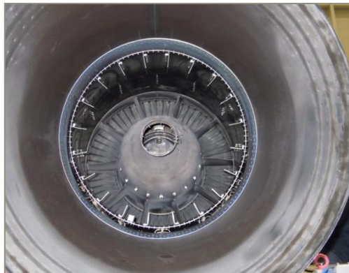
Figure 30. LFC installed on the A/C prototype.
