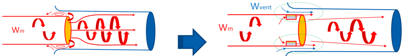
Figure 19: LFC effect on eductor operation (high swirl).
