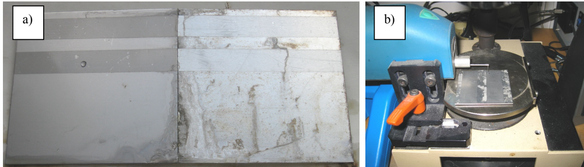
Figure 4: Corrosion couple stainless steel/aluminum (masked for the profile measurements) after the exposure (a), profilometer T1000 (b)
