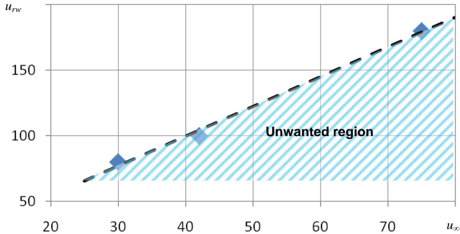
Figure 8: Dependence of the character reversed jet velocity  $u_{rw}$  from the counter flow velocity  $u_\infty$  for its reversing under air intake.
