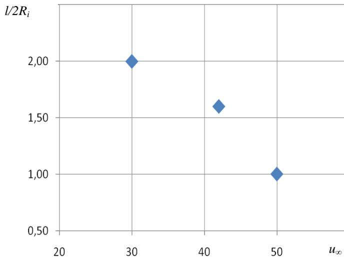
Figure 4: The dependencies of distance between engine inlet and reverse jet reversing point  $l$  from airplane velocities.  $R_i$  is a engine inlet radius.
