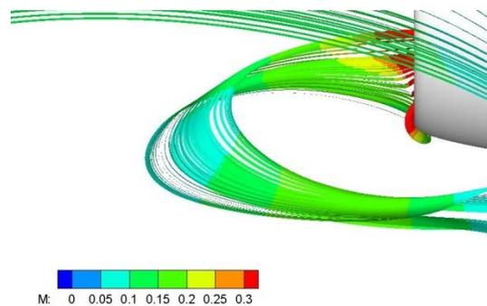
Figure 6: Flow lines for  $M_\infty = 0.1$ . Color is the Mach numbers distribution along flow lines.
