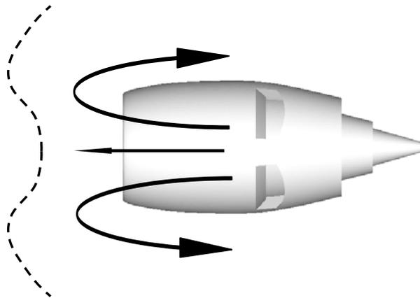
Figure 5: Scheme of reverse jets propagation. Solid line is a reverse flow and dashed line is a jet reversing zone.
