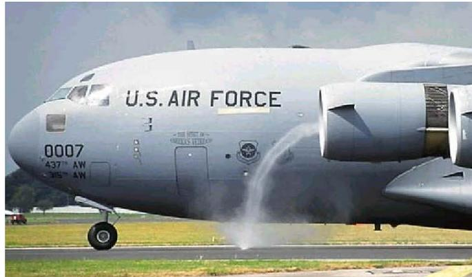
Figure 1: Photo of vortex flow at the engine inlet.
