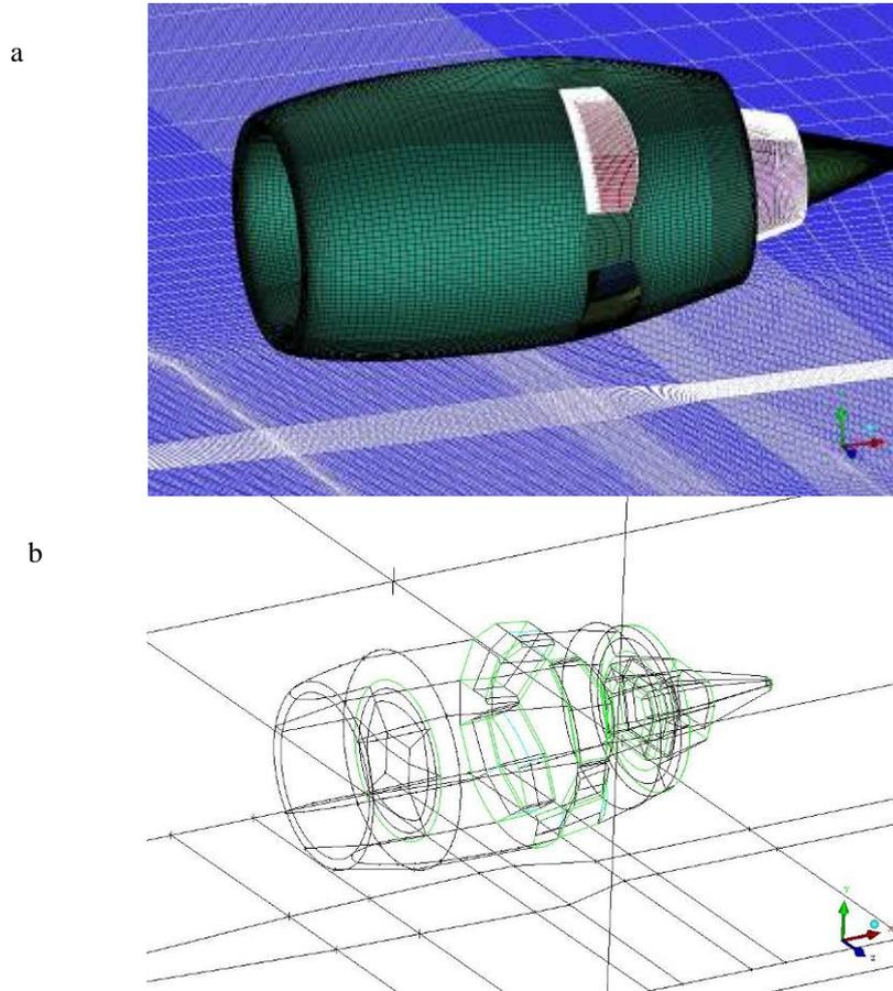
Figure 2: (a) – external view of pod and model of thrust reverse device;
