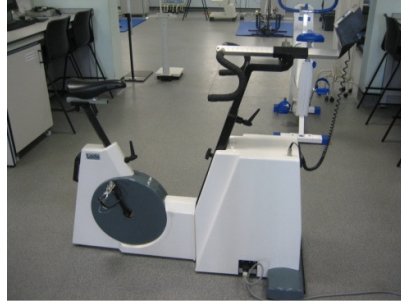
Figure 8: The facility dedicated to measuring the amount of power generated by human motion
