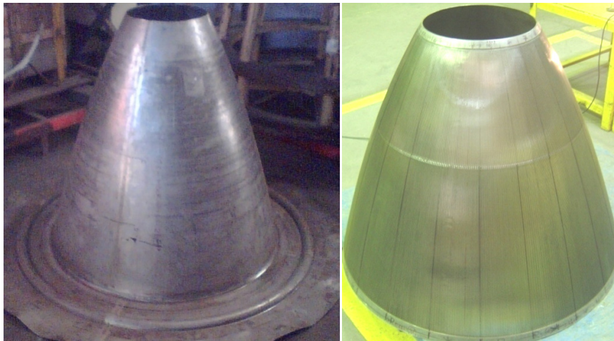
Figure.7 CE20 Nozzle after pressing and CUS channel milled nozzle
