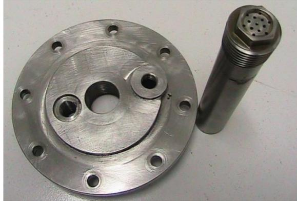
**Figure 4: Injection flange and the showerhead injector device**
