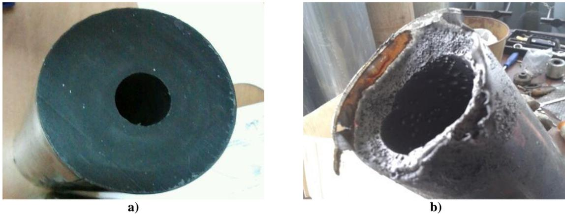
Figure 16: Detail of solid-wax grain burned in test SW\_05: a) before firing; b) after firing
