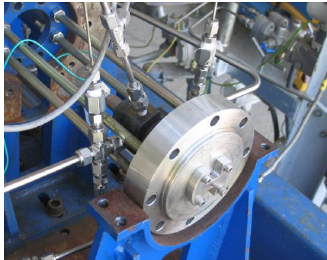
Figure 14 – Igniter mounted on test bench for leak testing
