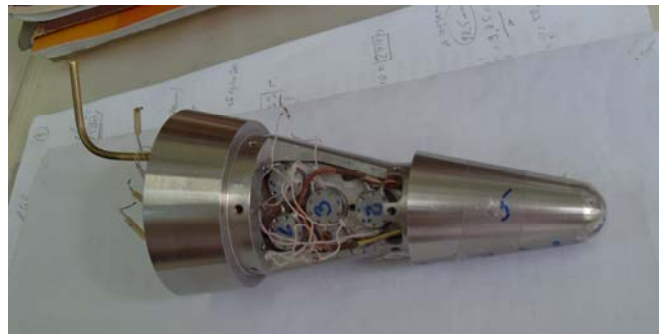
Figure 6. The model for pressure distribution measurement
