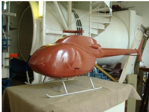
Figure 3: Wind tunnel model of the AKTAY helicopter fuselage.
