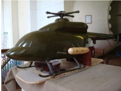
Figure 2: Wind tunnel model of the ANSAT-M2 helicopter fuselage.
