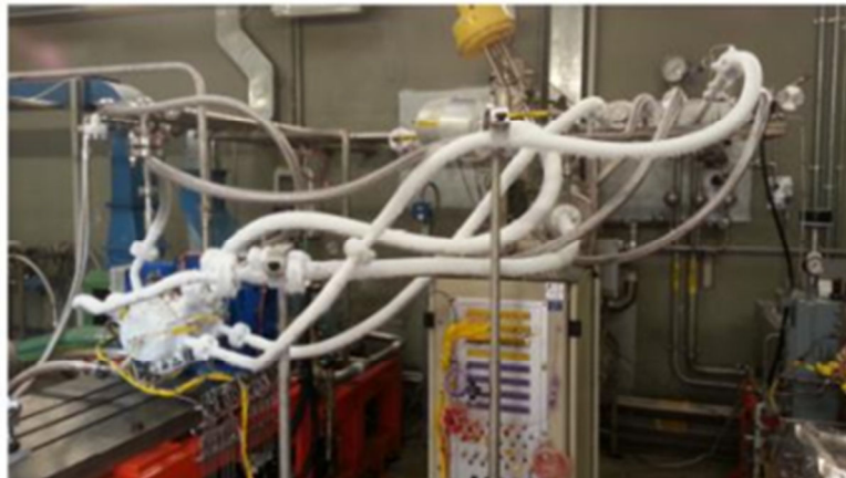
Figure 7: - LM10 MIRA bearing test rig in chill down conditions.
