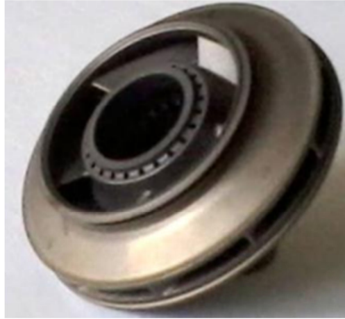
Figure 1: - LM10 MIRA CH4 pump impeller produced by DMLS technique.
