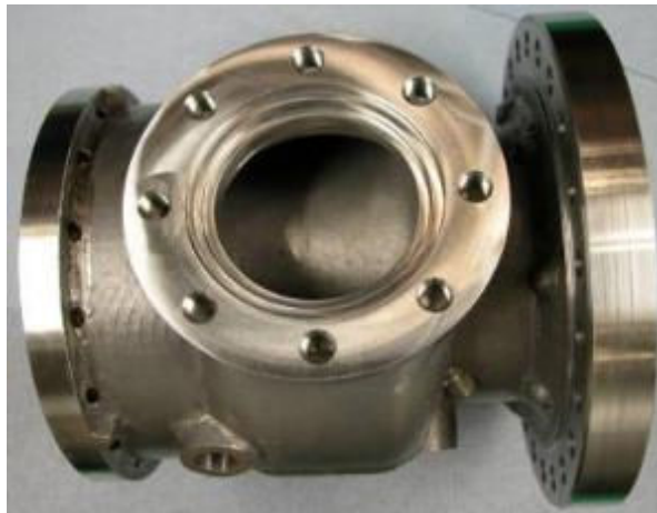
Figure 2: - LM10 MIRA CH4 turbine manifold produced by DMLS technic.
