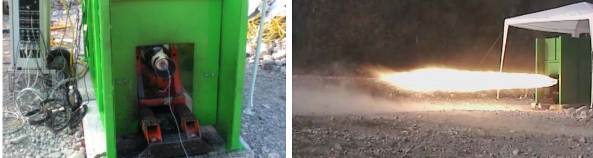
Figure 2 - CISAS open-air facility. This facility was used for the verification testing of the prototype motor. Each experiment was assembled/disassembled during the same test day, up to two tests/day.
