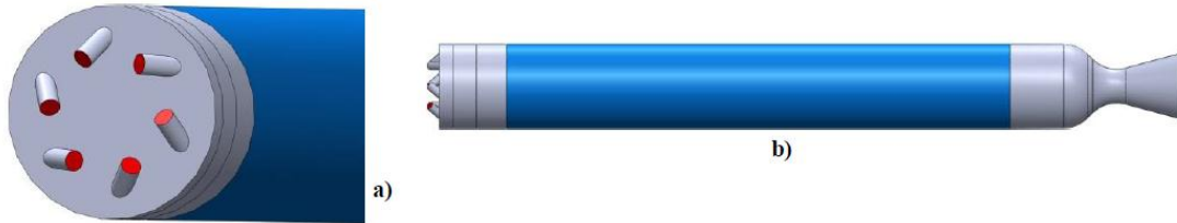
Fig.14 CFD geometry: a) injection details (red) and b) whole geometry with fuel injection (blue)
