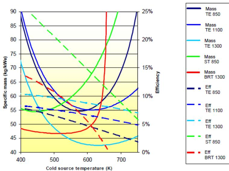
Figure 4: Balance of plant assessment (at 5kWe)
