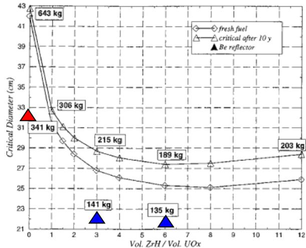
Figure 1: LuNPS-FPS by AREVA: concept (left)– Critical diameter vs moderator (right)
