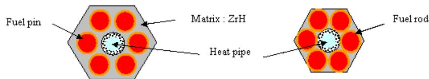
Figure 2: Fuel configuration: thermal on left (vol ZrH/vol UO<sub>2</sub>=2), fast on right
