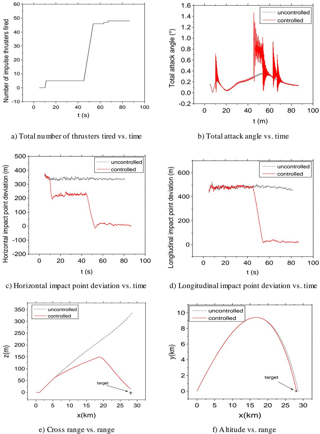
Figure 7: Correction performance of the optimum firing control scheme
