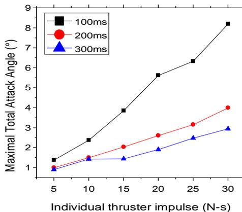
c) Maximal total attack angle vs. individual thruster impulse and minimum firing interval
