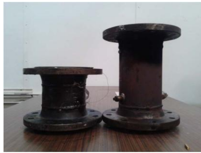
Figure 18 : Engine combustion chamber for the two design lengths
