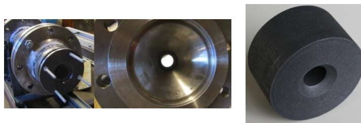
Figure 7: Graphite Con-Di nozzle and its support
