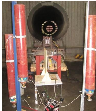
Figure 1: N 2 O Injection line
