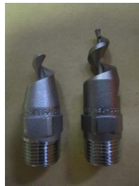
Figure 2: Full cone (left) and hollow cone (right) injectors
