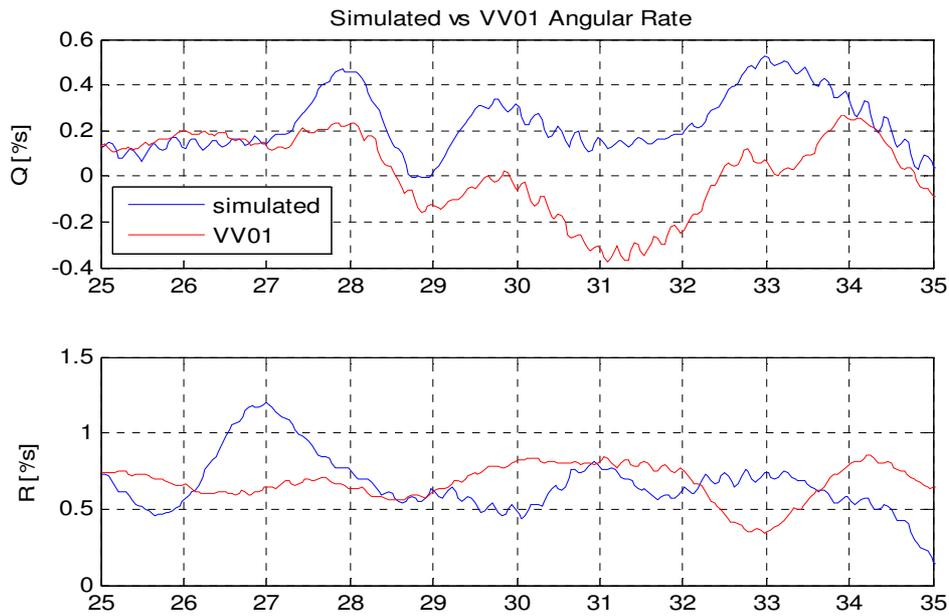
Figure 11: VV01 and simulated yaw and pitch rate from on board estimation (telemetry data)
