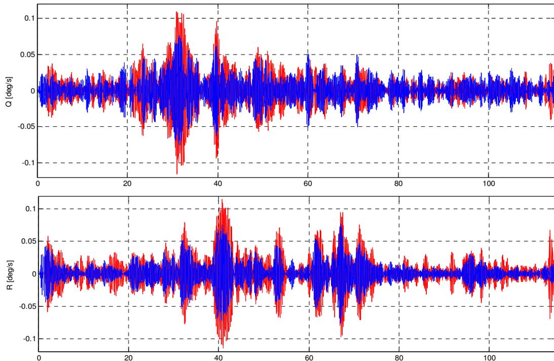
Figure 2: Signal in 4 Hz bandwidth (red: INS measurement; blue: LINS measurement)
