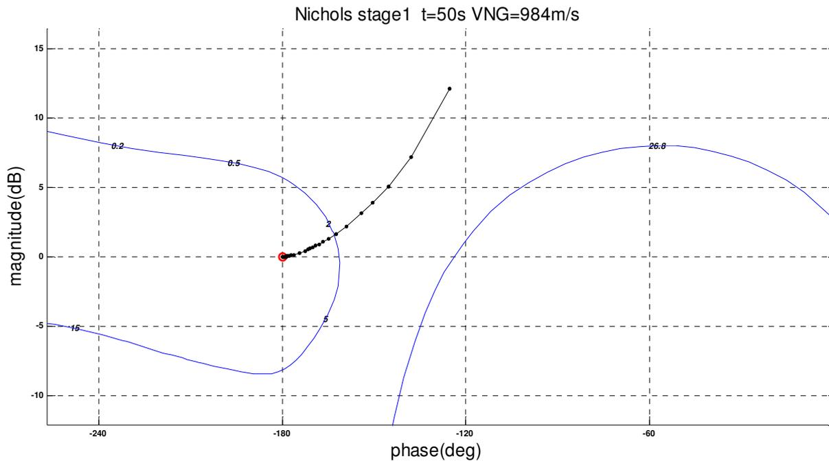
Figure 6: Nichols plot of the linear part and of the nonlinear part (backlash)
