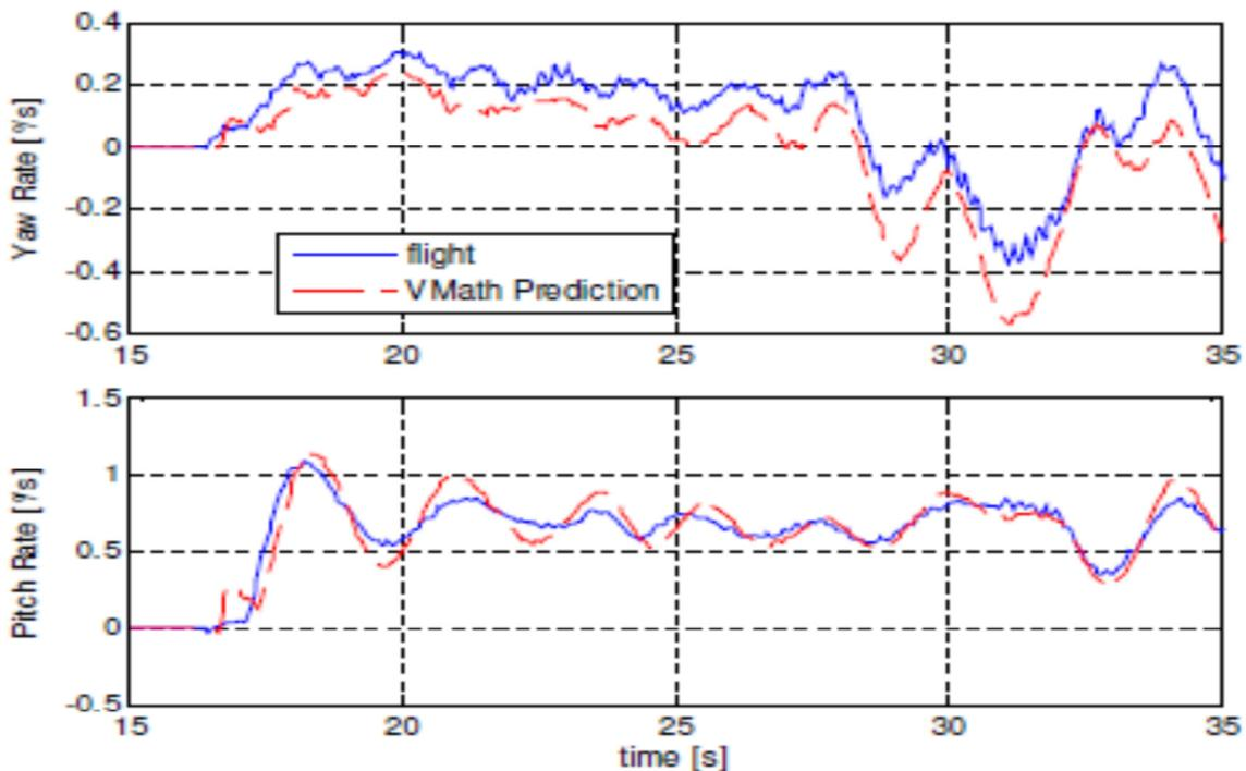
Figure 1: Comparison between Flight data and simulated reconstruction
