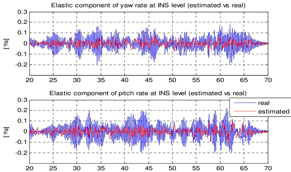
Figure 10: Real vs estimated elastic component of yaw and pitch rate at INS level
