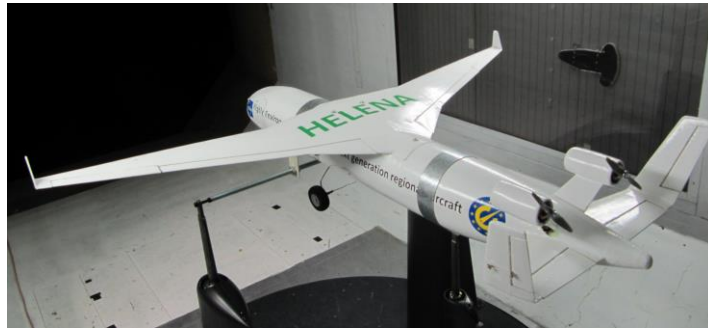
Fig 4. HELNA 1/20 scale flying mock-up in Wind Tunnel testing program
