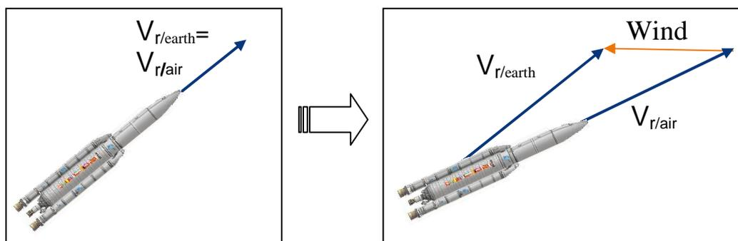
Figure 1.1: Gravity Turn For Trajectory Optimization Without (Left) And With (Right) Wind Biasing.
