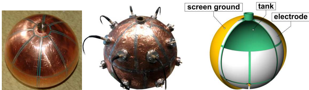
Figure 9: View of spherical capacitance sensor.
