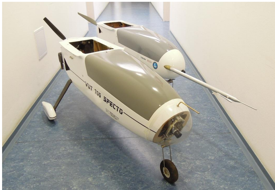
Figure 2: VUT 700 SPECTO and VUT 701 eSPECTO fuselages
