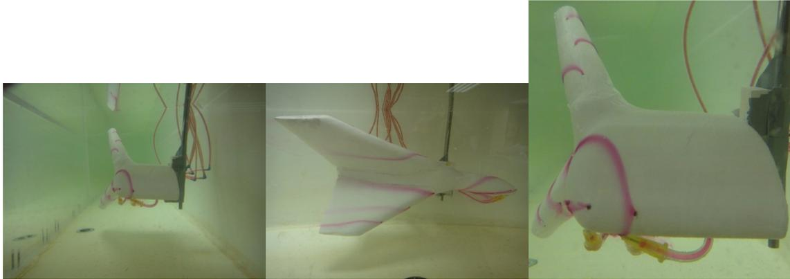
Figure 8: Winglet visualization.  $Re=1300$ ,  $\alpha=0^\circ$ ,  $\beta=5^\circ$ ,  $\phi=0^\circ$ .
