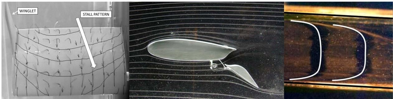
Figure 1: Several examples of visualization techniques carried out by the authors. From left to right, tufts in a zero sweep wing with winglet at  $20^\circ$  alpha, slotted flap in a smoke tunnel, and velocity profile in a hydrogen bubbles apparatus.
