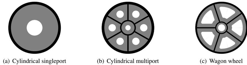
Figure 7: Solid fuel grain geometries
