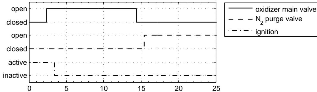
Figure 3: Valve and ignition control sequence
