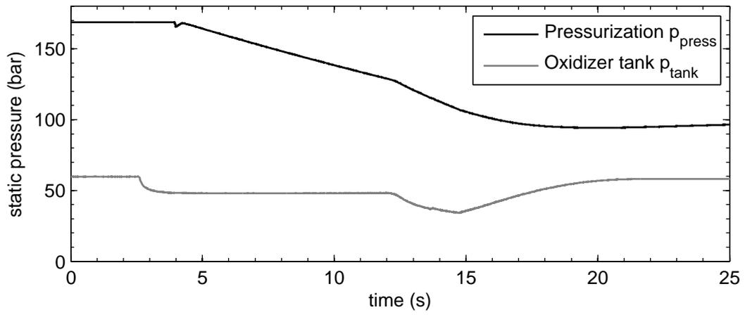
(a) Development of oxidizer supply pressures over time
