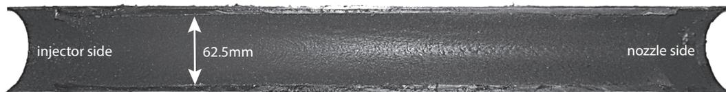
Figure 6: Opened HYPER1 grain after test
