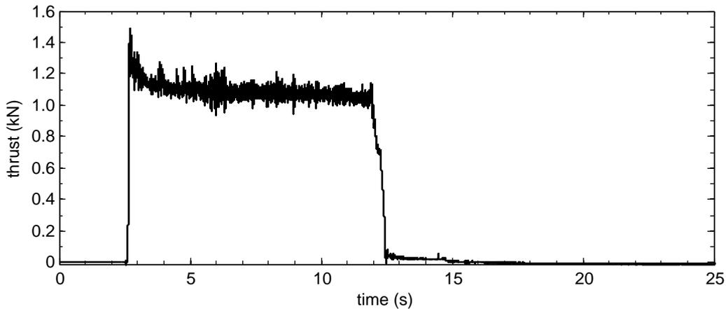
Figure 5: Development of thrust over time
