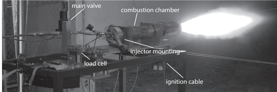
Figure 1: Snapshot from HYPER1 test video record
