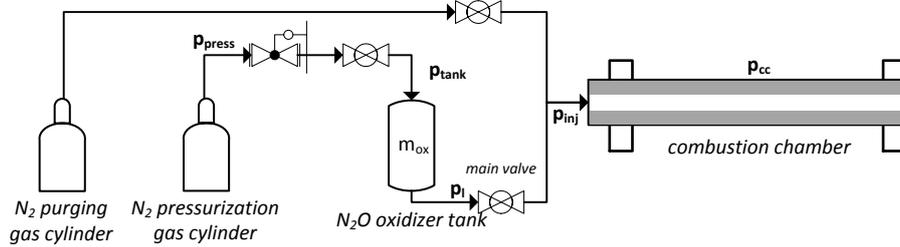
Figure 2: Simplified fluid plan of the test setup
