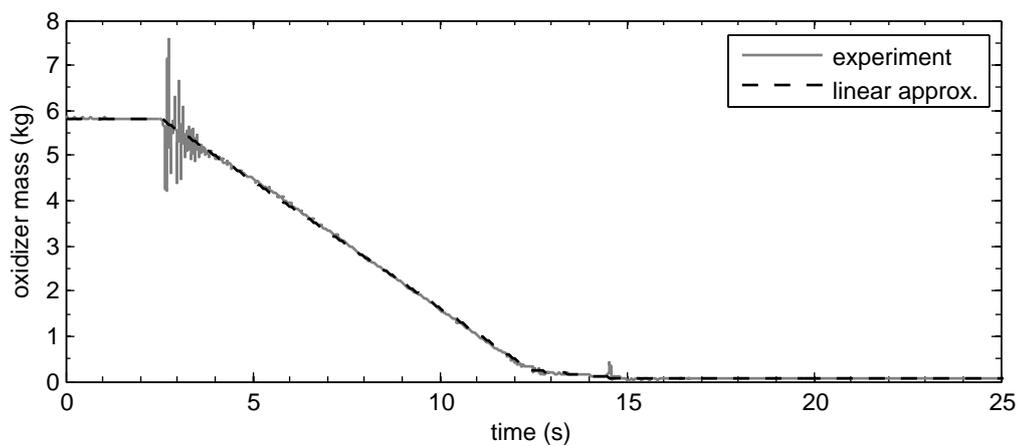
(c) Oxidizer supply mass development over time compared to linear approximation
