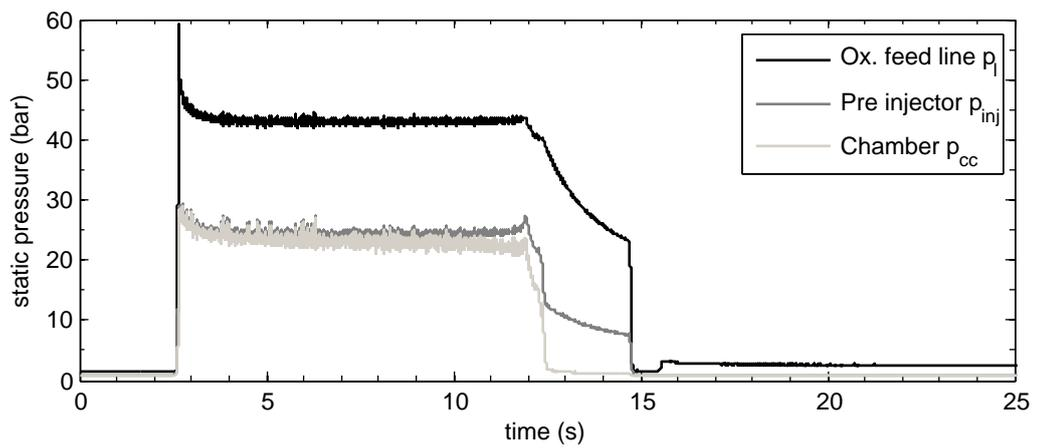
(b) Development of chamber, injector and feed line pressures over time
