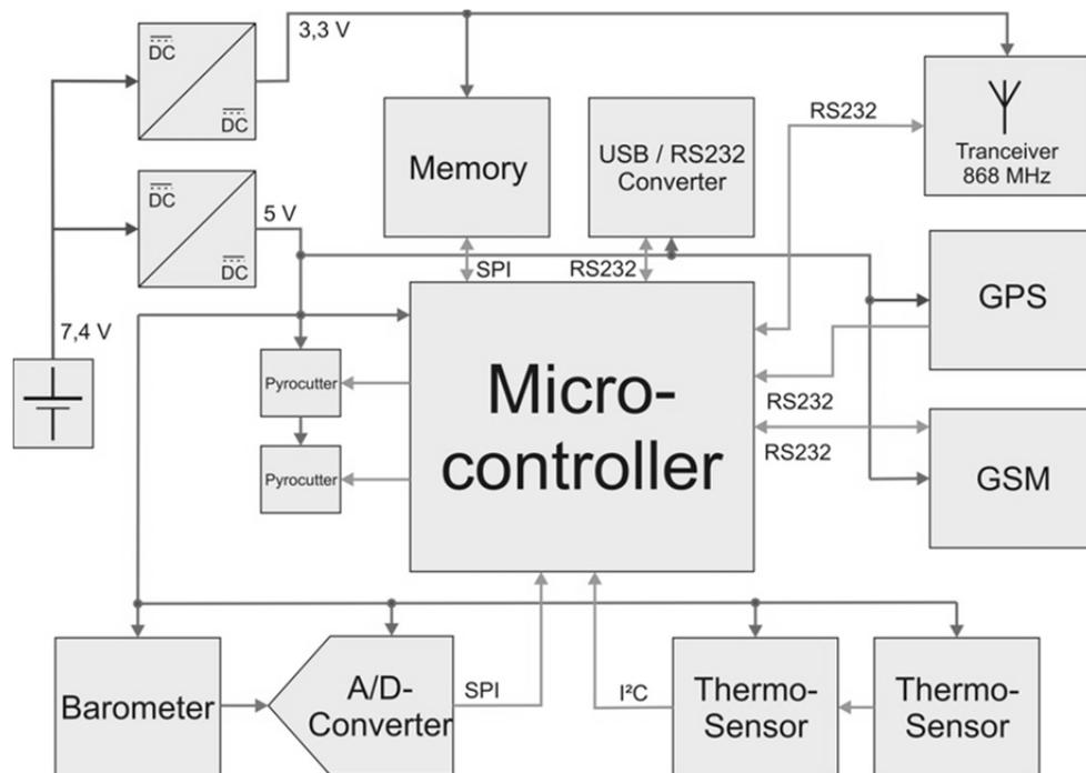
Figure 4: Architecture of the on-board computer of the payload box used during the launch campaign of research balloons
