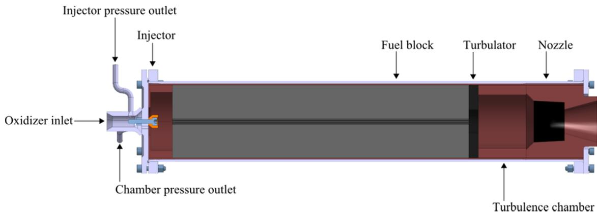
Figure 5: Sectional view of the HYDRA-3X
