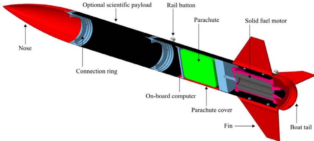
Figure 2: Sectional view of the research rocket Mephisto
