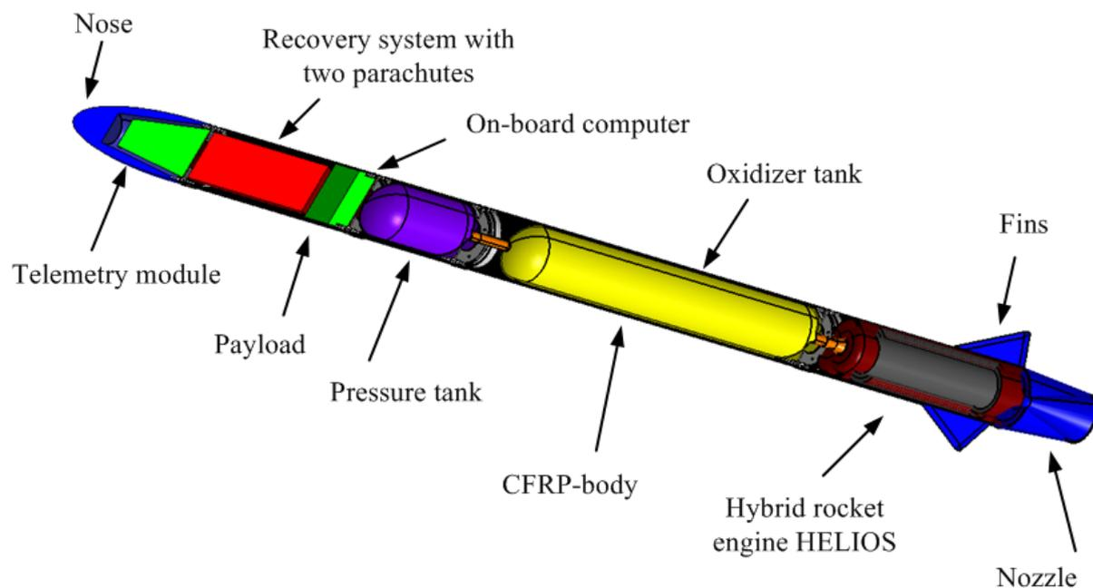
Figure 8: Sectional view of the pre-designed research rocket Regulus
