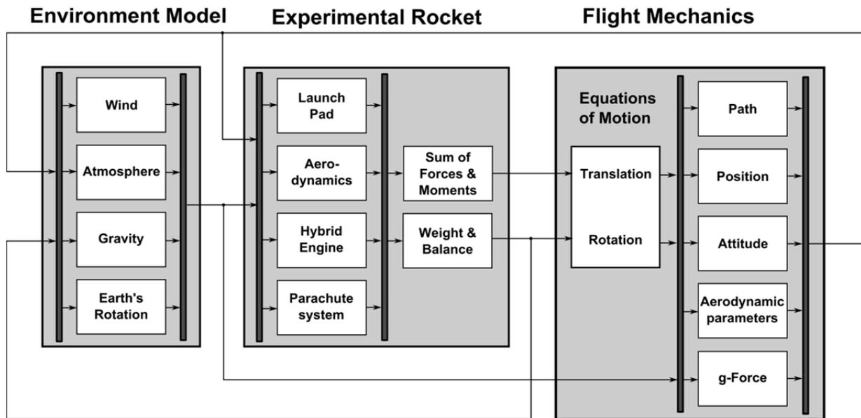
Figure 9: Architecture of the flight simulation ExRas
