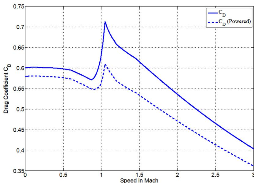
Figure 10: Drag coefficient vs. Mach number for the powered and unpowered rocket Regulus
