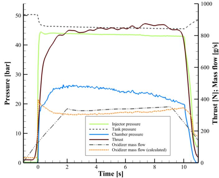
Figure 6: Diagram of measurements during the test run of the HYDRA-3X, which was conducted in October 2012
