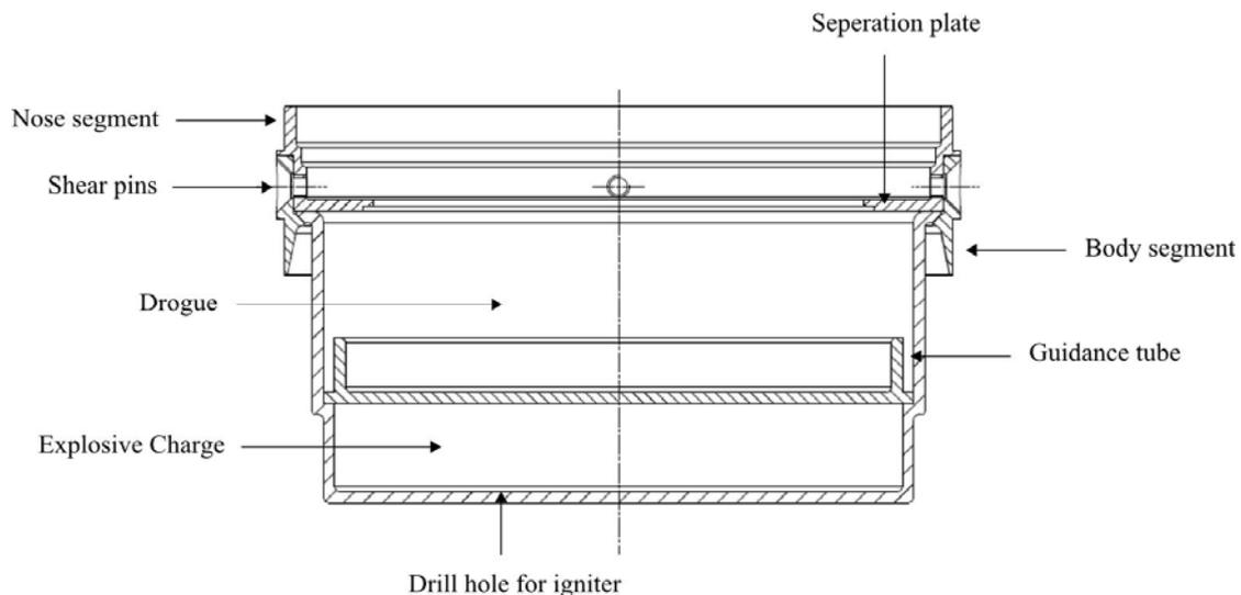
Figure 3: Sectional view of the separation system for the new recovery system
